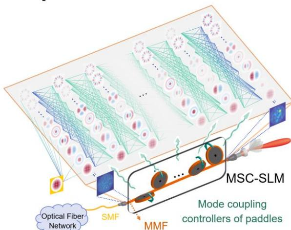
Figure 1 Principle of the proposed momentum space controlled spatial light modulators.
