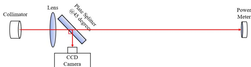
Figure 2. Experiment setup for observing the far-field beam profile and measuring the received optical power.
