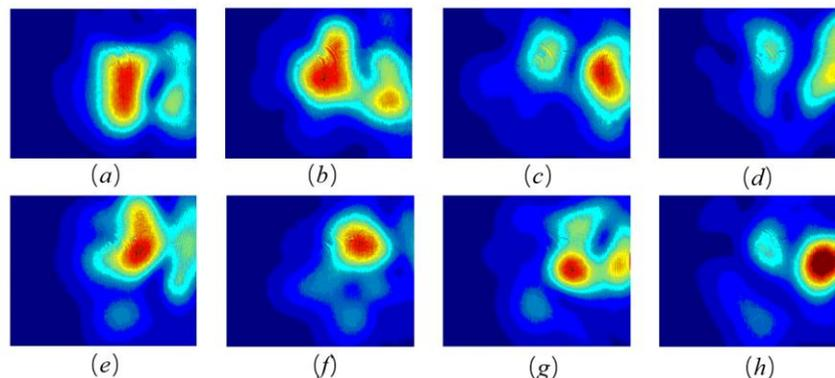
Figure 3. Measured beam profile of ITU C-band channels from C33 (1550.92nm) to C26 (1556.55nm).
