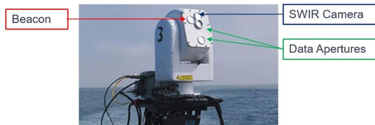
Figure 1. The APL optical terminal is housed in a General Dynamics Vector20 maritime gimbal. There are two bidirectional data apertures (simultaneous transmit and receive through both data apertures), a beacon aperture (transmit) and a camera aperture (receive) on the front of the gimbal.
