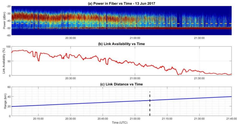
Figure 2. Data collected June 2017 in a ship to shore configuration; (a) One-second histograms of PIF compared to the receiver sensitivity (-44 dBm) in yellow; (b) One-second moving average link availability recorded by the retransmission system; (c) Distance between two terminals during the test run. 2 Gbps bidirectional data tested out to 30 km (black dotted line)
