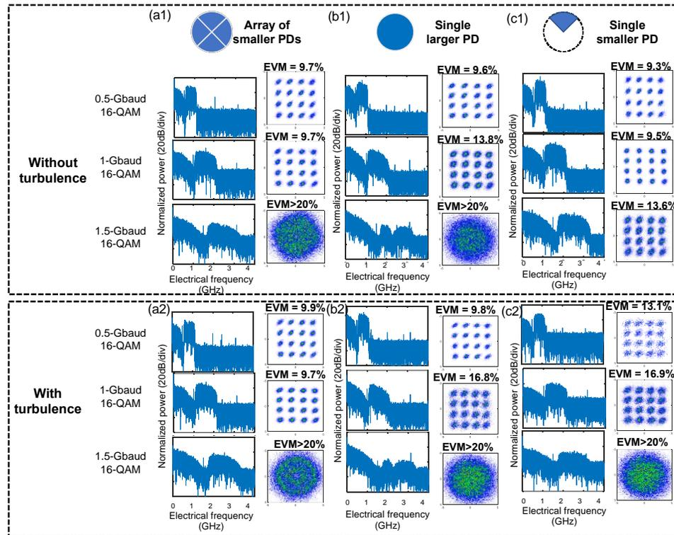
Fig. 4 Measured electrical spectra and recovered 16-QAM data constellations with different baud rates for different free-space PDs: (a1-a2) an array of smaller PDs, (b1-b2) single larger PD and (c1-c2) single smaller PD without and with turbulence effects. For (a2-c2), data in each row are measured under the same turbulence realization.
