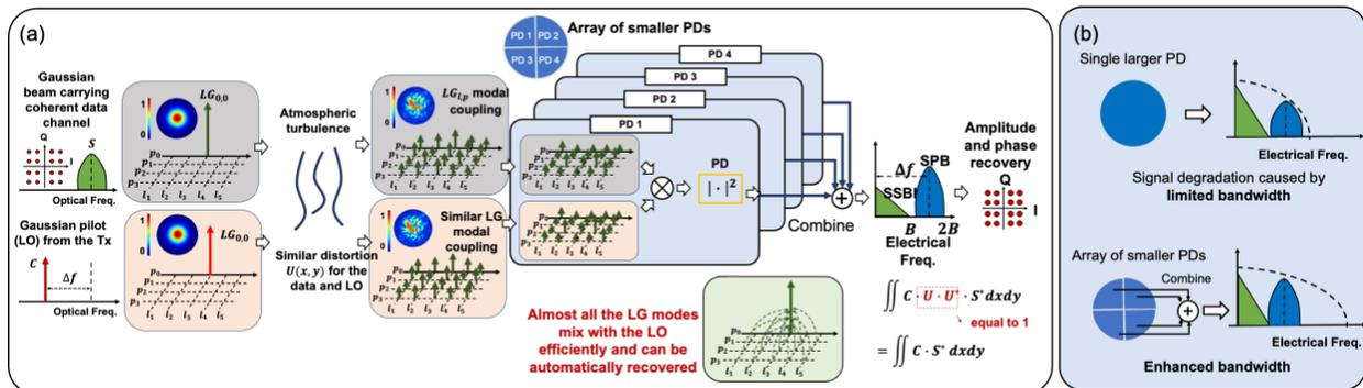
Fig. 1. (a) Concept of turbulence resilient self-coherent FSO communications using a pilot tone and an array of smaller photodiodes. (b) Concept of utilizing the array of smaller photodiodes for bandwidth enhancement. SSBI: signal-signal beating interference; SPB: signal-pilot beating.
