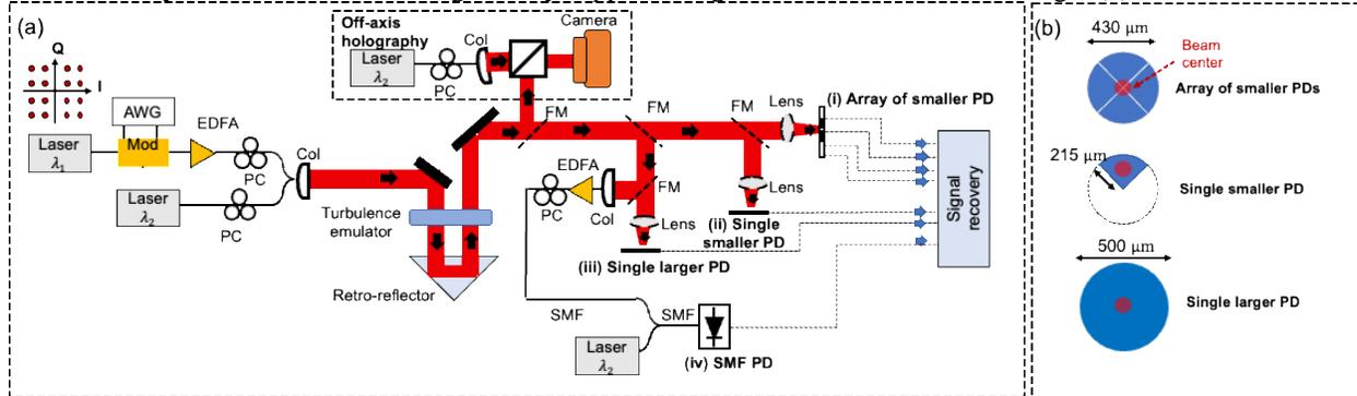
Fig. 2. (a) Experimental setup of an FSO link through emulated turbulence. AWG: Arbitrary Waveform Generator; EDFA: Erbium-doped Fiber Amplifier; PC: Polarization Controller; ; FM: flip mirror; SMF: single-mode fiber; DSP: Digital Signal Processing. (b) Size of the free-space PD used in our experiment. For the array of smaller PDs and single smaller PD, a PX00M3 quadrant InGaAs PD from Albis is used. For the single larger PD, a Thorlabs FDGA05 InGaAs PD is used.
