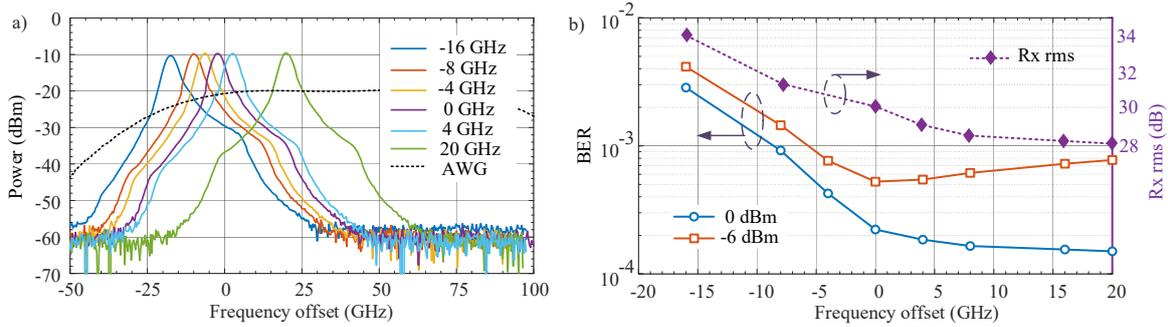
Fig. 2a) Optical spectra of 100 Gb/s DMT signal after AWG with various values of frequency offset related to the optimum DML frequency; b) – BER and Rx signal rms as the function of frequency offset (relative to the optimum DML frequency) in the B2B case
