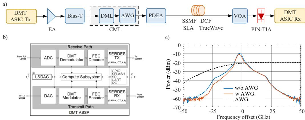
Fig. 1a) Experimental setup; b) – Basic block diagram of the 100 Gb/s DMT ASIC; c) – Optical spectra of modulated DMT signals with and without the AWG; The center wavelength is 1312.9 nm. DSP – digital signal processing; EA – electrical amplifier; VOA – variable optical attenuator; PDFA – O-band optical amplifier
