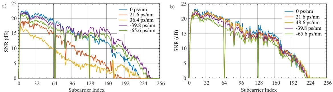
Fig. 3a) Measured SNR versus subcarrier index for 100 Gb/s DMT transmissions with conventional DML (w/o AWG); b) – Measured SNR versus subcarrier index for 100 Gb/s DMT transmissions with CML (with AWG)
