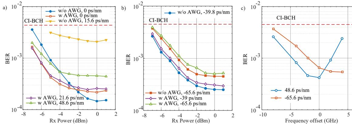
Fig. 4a) Sensitivity measurements for 100 Gb/s DMT transmissions with DML and CML in positive dispersion regime ; b) – Sensitivity measurements for 100 Gb/s DMT transmissions with DML and CML in negative dispersion regime; c) – Frequency offset tolerance for CML-based transmission at 0 dBm of Rx optical power
