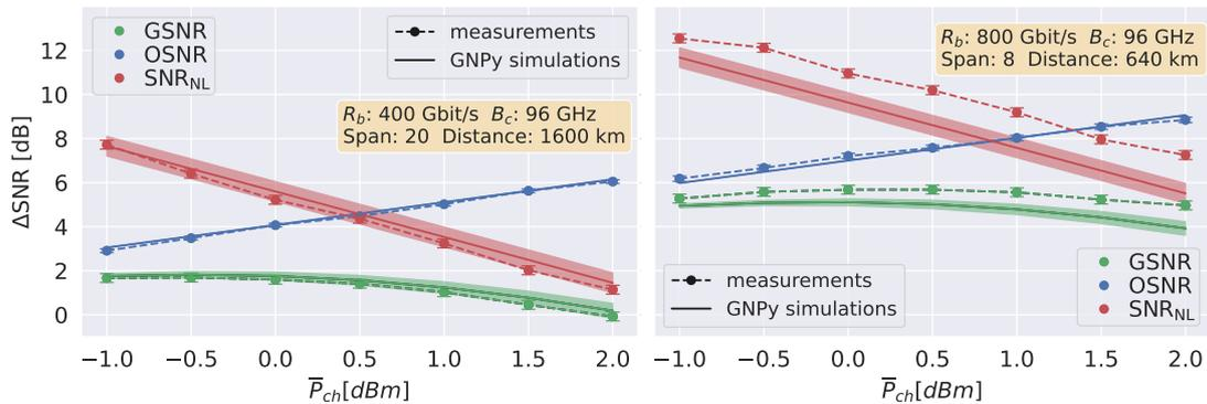
Fig. 2: Power sweeps for two selected bit rates. The shaded area surrounding the solid lines represents the variation of the GSNR and  $SNR_{NL}$  predictions varying the connector loss within a 0.5 dB range.
