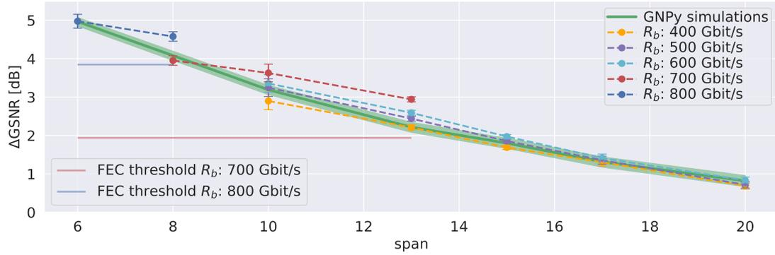
Fig. 3: Measured and simulated GSNR at different receiving distances for all the investigated bit rates. The FEC thresholds of the  $R_b$  lower than 700 Gbit/s are not shown in the figure as they are not significant being lower than the minimum GSNR reached after 20 spans of transmission.
