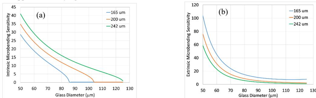
Fig. 2 Calculated microbending sensitivity (a) intrinsic (b) extrinsic.
