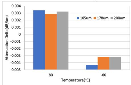
Fig. 3 Attenuation changes at two temperatures on loose coiled fibers.
