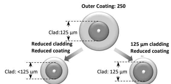
Fig. 1 Two approaches for reducing fiber diameter.
