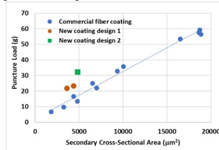
Fig. 4 Coating puncture resistance test results.
