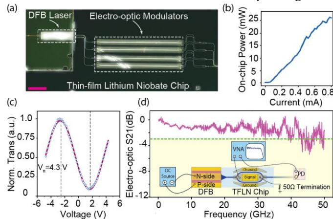
Fig.2 (a) Micrograph image of the integrated DFB-TFLN laser-transmitter. (b) Measured LI curve for the device shown in (a). (c) Measured  $V_{\pi}$  (d) electro-optic response of the integrated transmitter ( $S_{21}$ )
