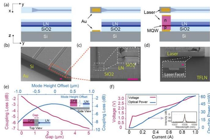
Fig. 1. (a) Fabrication Steps for integration of DFB Laser on TFLN Platform (b) SEM images of the fabricated recessed region and the bonded laser. (c) Simulation results for coupling loss vs the gap and mode-height offset between the laser and the TFLN waveguide, (d) LIV curve for the laser bonded to the passive TFLN circuits.
