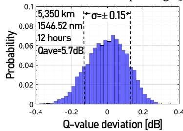
Fig. 4. Histogram of Q-value deviation during 12 hours UC-MCF cable transmission
