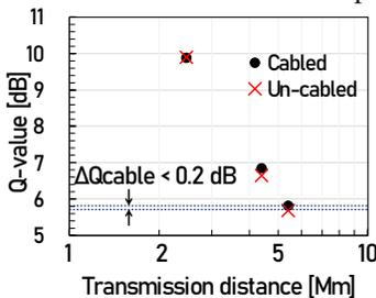
Fig. 3. Measured Q-value of cabled and un-cabled UC-MCF transmitted signal
