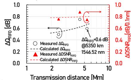
Fig. 5. Q-value and OSNR change by the reduction of the number of FIFO and UC-MCF splice point
