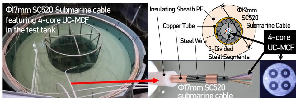
Fig. 1. Fabricated submarine cable prototype featuring 4-core UC-MCF
