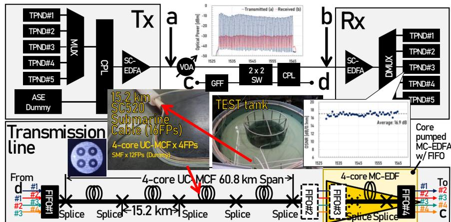
Fig. 2. Experimental-setup using 4-core MCF submarine cable prototype and 4-core MC-EDFA with and without FIFO
