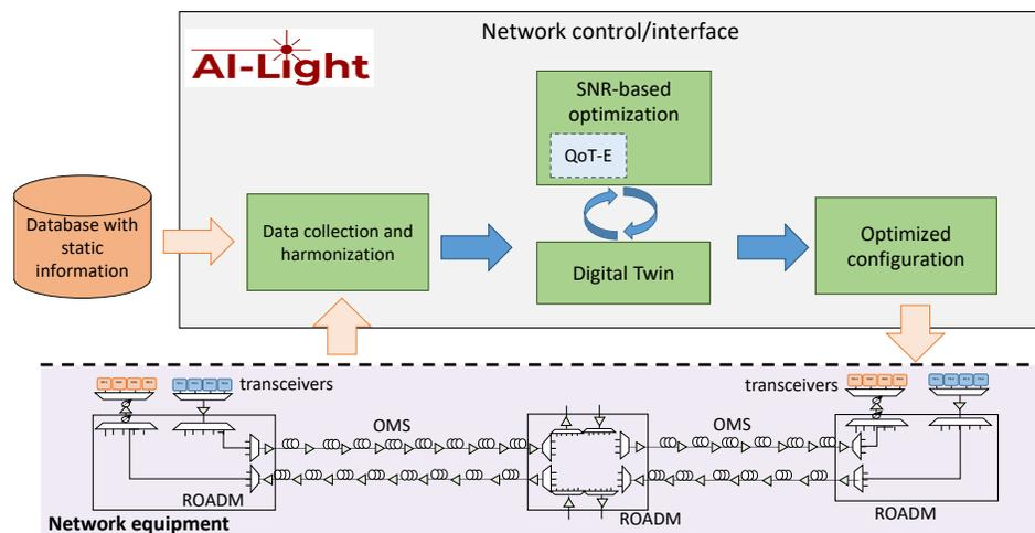
Fig. 2: structure of the demo: (top) AI-Light SDN framework; (bottom) network equipment.
