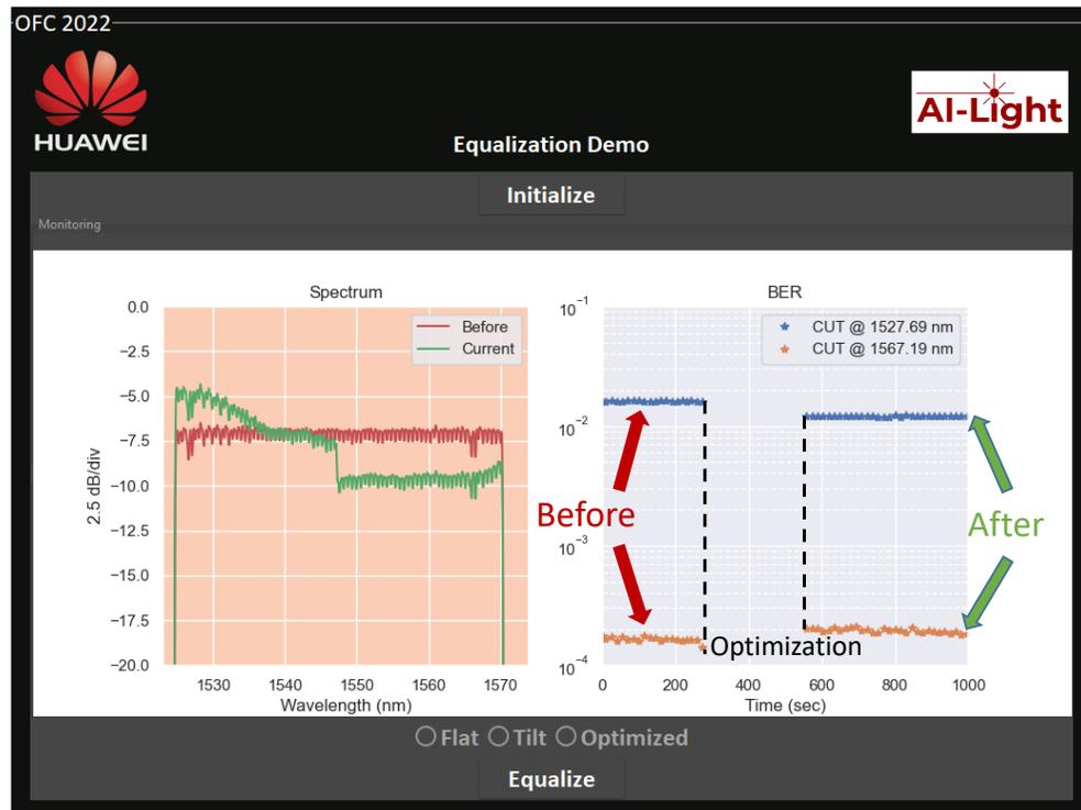
Fig. 3: GUI showing the monitored spectrum and the BER over time before (left) and after (right) the optimization
