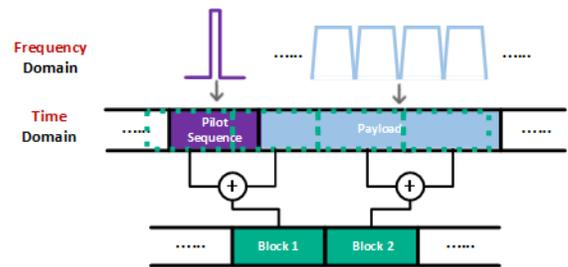
Fig.2 New optimized method of finding the rough place of FrFT
