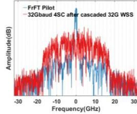
Fig 11. The 32Gbaud 4SC frequency spectrum at the receiver of experiments
