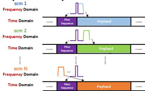
Fig. 1: Structure of FrFT-DC Pilot of Digital SCM
