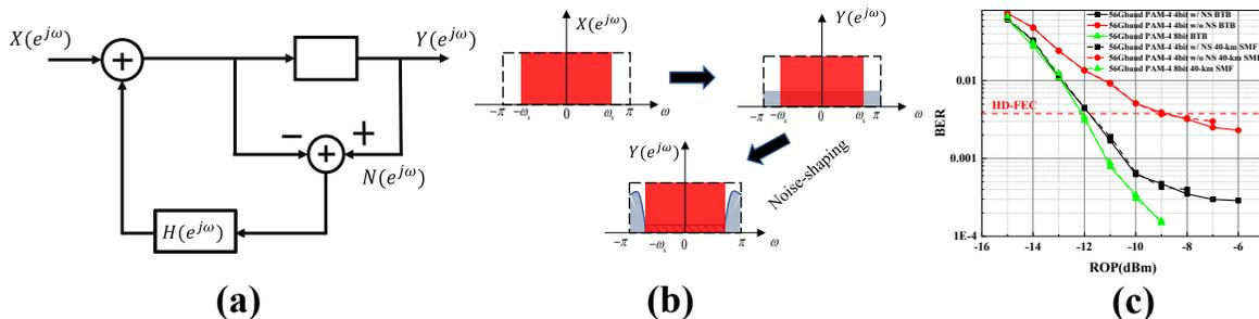
Fig. 1. (a) Linear models of noise shaping technique. (b) Operating principle of noise shaping technique in frequency-domain. (c) BER versus ROP of 56 Gbaud PAM-4 in OBTB and 40 km SMF transmission.
