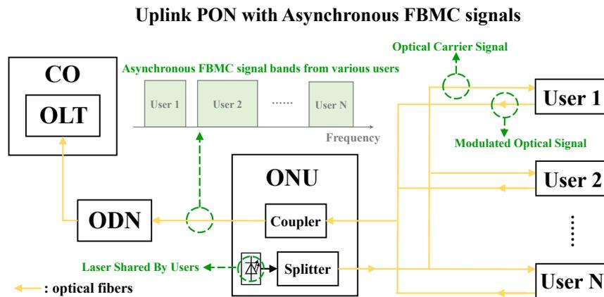
Fig. 3. A flexible laser sharing PON uplink scheme based on FBMC.
