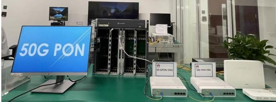
Figure. 1: real-time 50G-PON prototype in the form of commercial chassis
