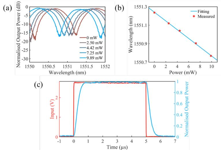
Fig. 3. (a) Normalized output power from the aMZI under different driving powers. (b) The wavelength shifts of the interference dip of the modulator with the heating power. (c) Dynamic response of the aMZI.
