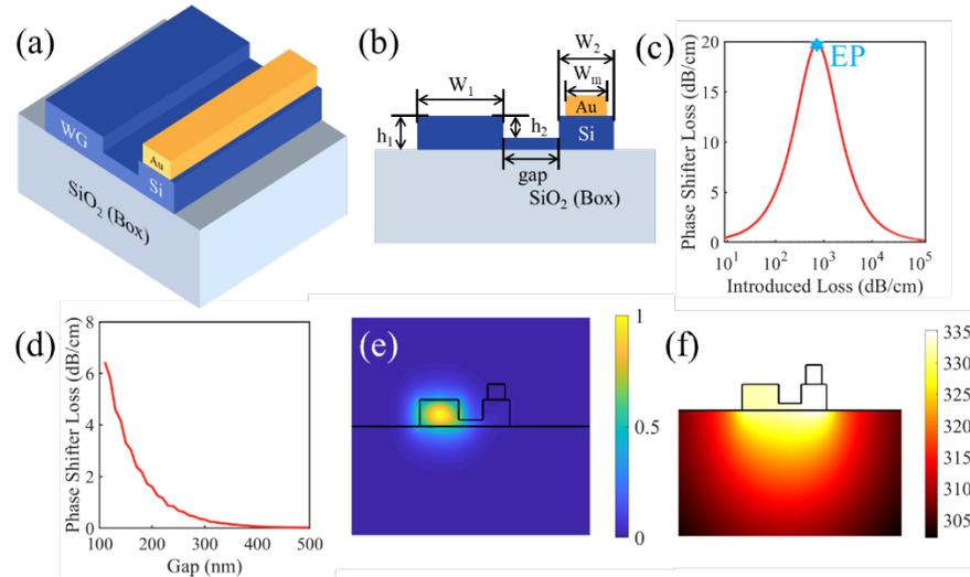
Fig. 1. Schematic (a) and cross-section view (b) of the proposed phase shifter.  $W_1=500$  nm,  $W_2=300$  nm,  $W_m=300$  nm,  $gap=300$  nm,  $h_1=220$  nm,  $h_2=150$  nm. Calculated loss of the proposed phase shifter under different introduced losses on the right thin waveguide (c) and different gaps (d). (e) Simulated optical mode profile inside the phase shifter. (f) Simulated temperature distribution of the phase shifter at a driving power of 7.9 mW.
