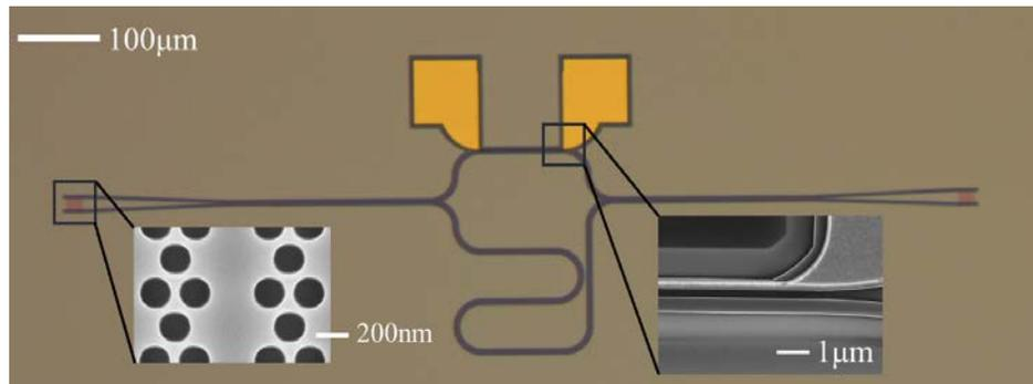
Fig. 2. Optical image of the aMZI. Inset shows the zoom-in SEM images of the photonic crystal grating coupler (left) and the phase shifter (right).
