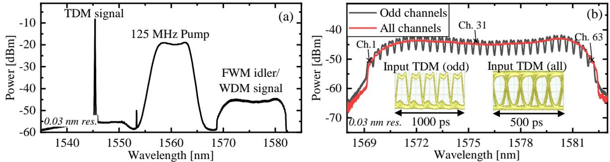
Fig. 2. (a) FWM spectrum showing input TDM signal, pump and resulting WDM signal. (b) WDM spectra after pump suppression for all channels and odd channels respectively. Insets show the TDM waveforms before conversion.
