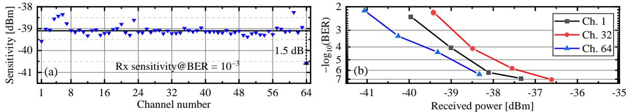
Fig. 4. (a) Received power sensitivity at  $\text{BER} = 10^{-3}$  for all channels. Black line indicates the mean, and the difference from the best channel (64) to the mean sensitivity is indicated to be 1.5 dB. (b) BER vs. received power curves for representative WDM channel wavelengths.
