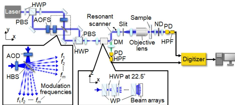
Fig. 2. Schematic of the FTDM single-pixel imaging setup. The left inset shows the details of generating a pair of intensity-modulated beam arrays from acousto-optic deflectors by optical interference. HWP, half-wave plate; PBS, polarizing beam splitter; AOFS, acousto-optic frequency shifter; AOD, acousto-optic deflector; HBS, non-polarizing half beam splitter; WP, Wollaston prism; DM, dichroic mirror; ND, neutral-density filter; PD, photodetector; HPF, high-pass filter.
