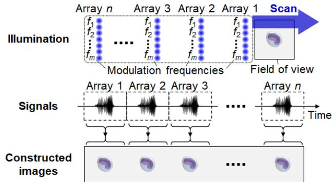
Fig. 1. Concept of FTDM single-pixel imaging.
