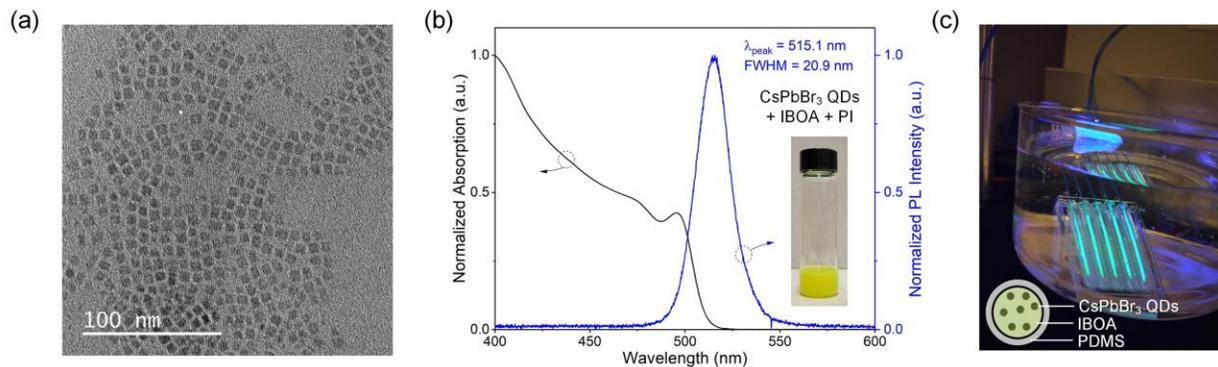
Figure 1. (a) TEM image of the CsPbBr<sub>3</sub> QDs. (b) Normalized absorbance and photoluminescence spectra of CsPbBr<sub>3</sub> QDs in IBOA and PI solution. (c) An array of perovskite-based scintillating fibers optical receivers submerged in a water bath. The inset illustrates the core and cladding layers of the as-fabricated scintillating fibers.
