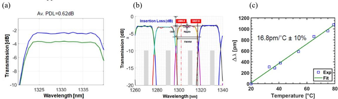
Fig.4 Polarization and Temperature dependence of PIC (a) Polarization independent loss of optical transmission loss (b) The optical spectrum of DEMUX in the wavelength range of 4ch CWDM (c) Wavelength shift of CWDM passband as a function of temperature
