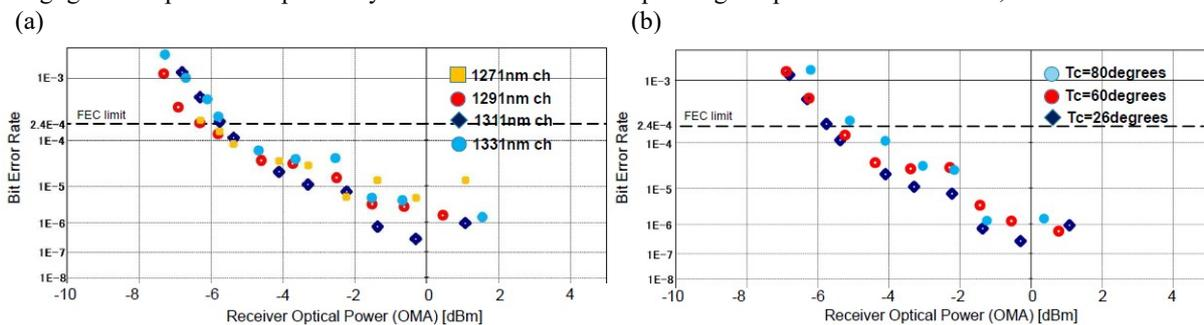
Fig.6 (a) BER for ROSA of all output channels (b) Temperature dependency for BER at 26°C, 60°C and 80°C
