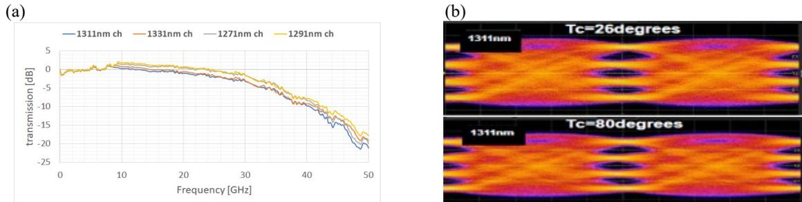
Fig.5 (a) Bandwidth of ROSA (b) Output waveform eye diagrams of ROSA at the case temperature ( $T_c$ ) of 26°C and 80°C for 53.125 Gbaud PAM4 signals
