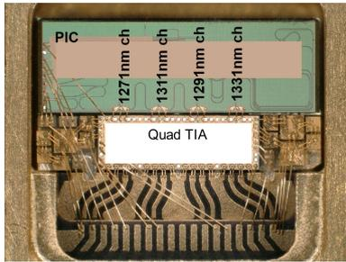
Fig.2 Photograph view of ROSA package inside including PIC and Quad TIA
