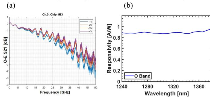
Fig.3 Optical Characteristics of the Ge photodiode in PIC (a) Frequency response (b) Responsivity on O-band
