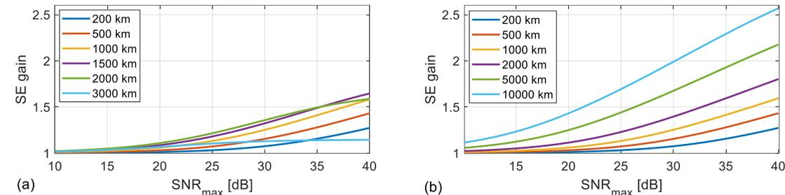
Fig. 5. SE gain over an ideally amplified SMF system for an ideal NANF system using (a) a single unamplified span and (b) 100-km lumped amplification spans as a function of maximum transponder SNR at different transmission distances.
