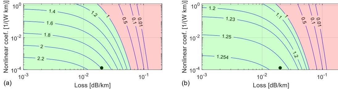
Fig. 3. SE gain over an ideally amplified SMF system for an unamplified single-span NANF system (a) without and (b) with 30-dB noise floor.
