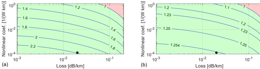
Fig. 4. SE gain over an ideally amplified SMF system for a lumped-amplified NANF system (a) without and (b) with 30-dB noise floor.
