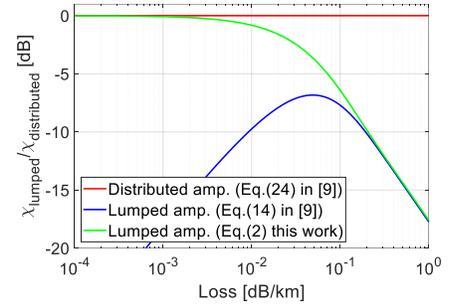
Fig. 2 Normalized noise coefficient.
