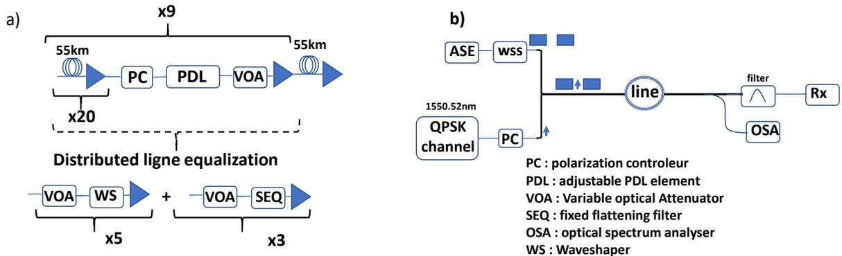
Fig.2(a): line description, (b) emitter and receiver
