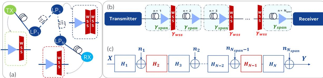
Fig.1(a): Simplified multi-point submarine link with different landing point (LP). (b): System model assumed for analytical study (c) its equivalent mathematical model
