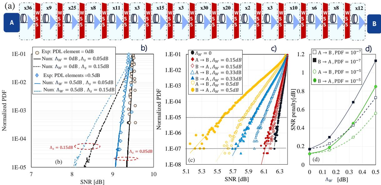
Fig.3(a): submarine line used for simulation of figure 3c) and 3d) (b) experimental and numerical SNR distribution for line used in experiment of Fig2, (c), (d) numerical SNR distribution for propagation in both directions for different values of  $\Lambda_w$  (d) SNR penalty versus  $\Lambda_w$  at outage probability of  $10^{-5}$  and  $10^{-7}$
