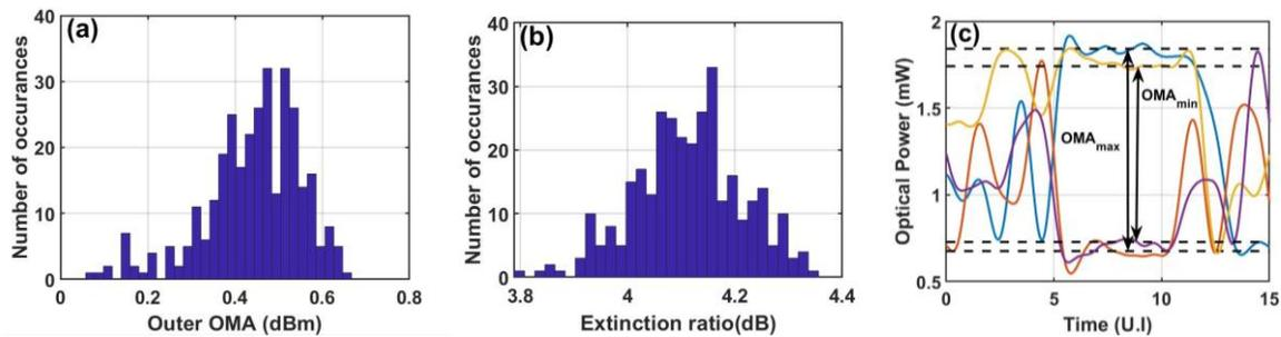
Fig 3. (a) Outer OMA spread (b) Extinction ratio spread (c) sub-patterns for highest and lowest outer OMA
