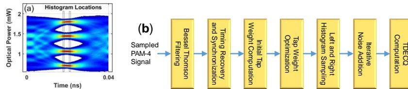
Fig 1. (a) Experimental 25GBaud equalized eye (b) Block diagram of TDECQ algorithm implementation
