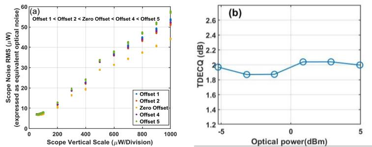
Fig 6. (a) Variation of scope noise for various settings (b) TDECQ variation with launch power for accurate noise characterization
