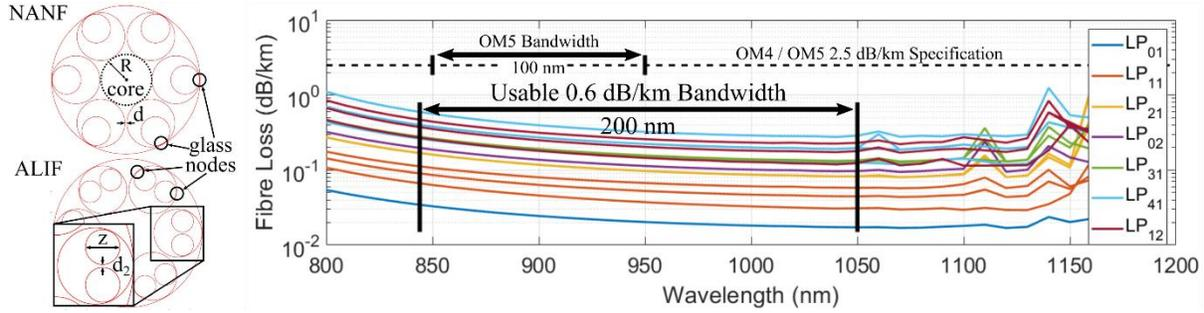
Fig. 1: A comparison of the NANF (top-left) and ALIF (bottom-left) structures and the loss spectrum of the 10-element multimode ALIF geometry shown in Fig. 2. In the ALIF, careful choice of the nested tube diameter  $z$  and their separation distance  $d_2$  allows control of the loss and modal content of the fibre.
