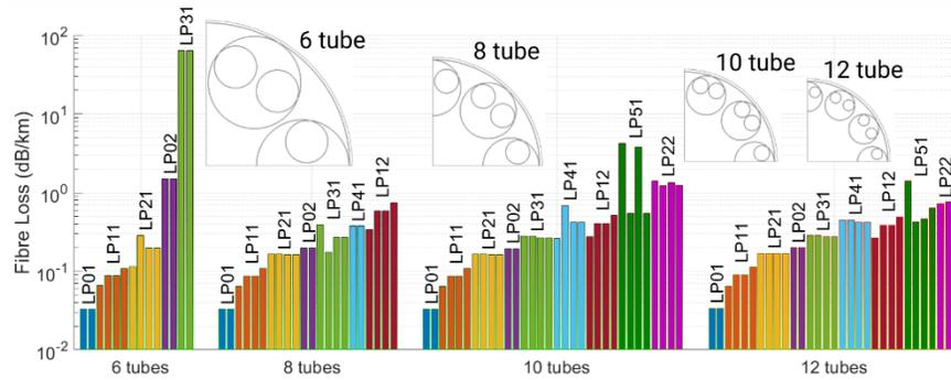
Fig 2: Losses of the core guided modes of the shown fibre geometries. The core diameter and tube wall thickness of every fibre is  $50\ \mu\text{m}$  and  $330\ \text{nm}$  respectively.
