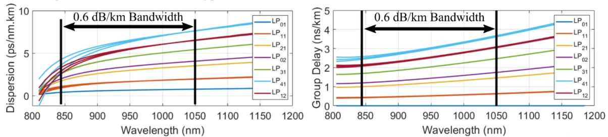
Fig. 3: The DGD (left) and chromatic dispersion (right) of the 10 tube fibre shown in Fig. 2.
