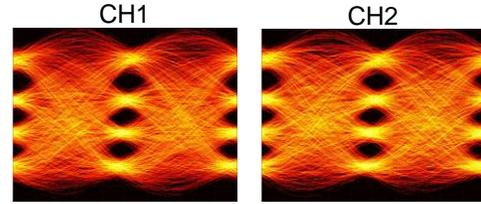
Fig. 3. 2km-transmission 53-Gbps/ch PAM4 eye diagrams after FFE.
