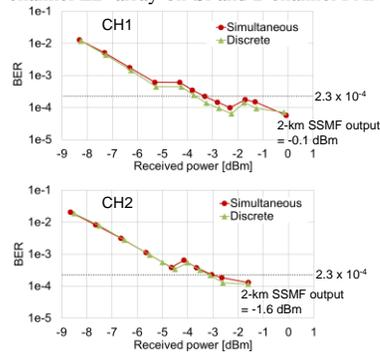
Fig. 4. Measured BER dependence of received power for discrete and simultaneous operation over 2-km-long SSMF.
