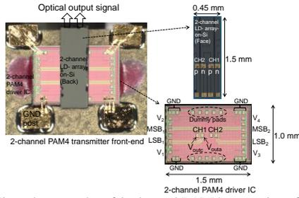
Fig. 2. Microphotographs of 2-channel PAM4 transmitter front-end (left) and the 2-channel LD-array-on-Si and 2-channel PAM4 driver IC (right).
