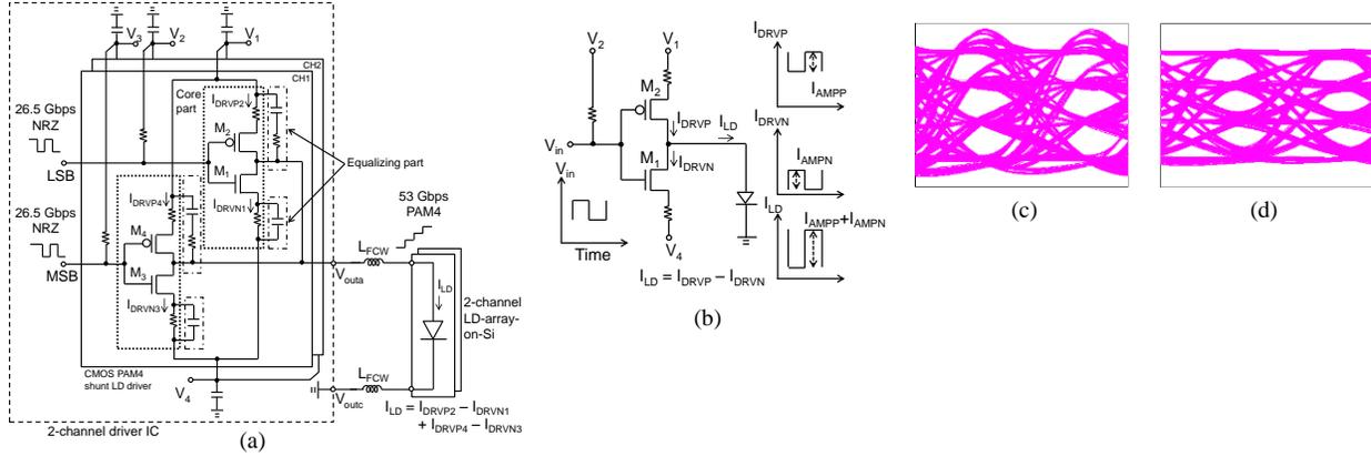
Fig. 1. (a) Block diagram of 2-channel PAM4 transmitter front-end. (b) Operation of core parts. Simulated 53-Gbps/ch PAM4 optical output waveform for simultaneous operation (c) without equalizing part and (d) with equalizing part.
