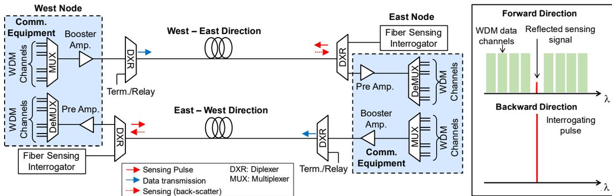
Fig. 1. Bidirectional dual-usage architecture, where data transmission and distributed fiber-optic sensing coexist on different wavelengths. The sensing and data signals counter-propagate in each optical fiber to reduce their nonlinear interaction.
