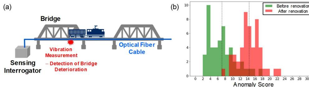
Fig. 4. (a) Bridge structural health monitoring using DFOS, (b) ML classification of bridge health showing distribution of “Anomaly score” before and after renovation.
