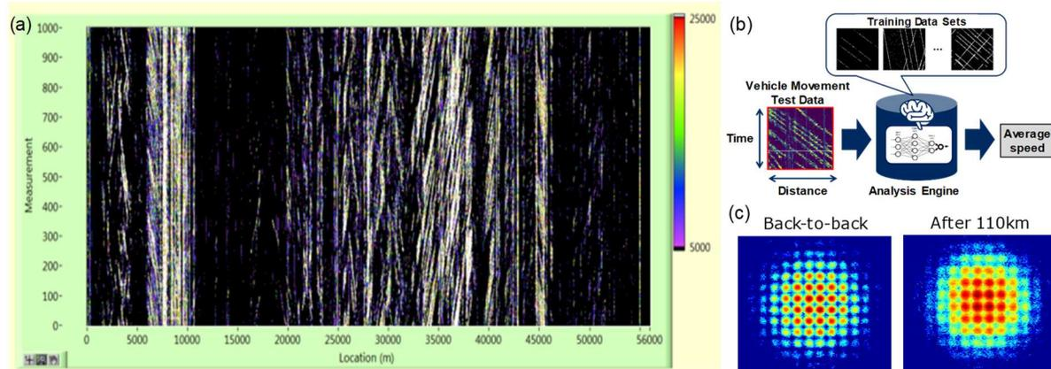
Fig. 3. (a) “Waterfall” plot showing vehicular traffic pattern, (b) Machine learning to determine vehicular direction and average speed, (c) Constellation diagrams of PS-144QAM channels which counter-propagated against the DFOS system.
