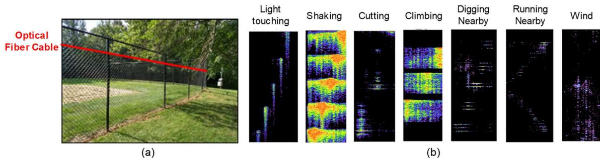
Fig. 2. (a) DFOS system mounted on a fence, (b) “Waterfall” plots for different vibration events which can be classified by machine learning.
