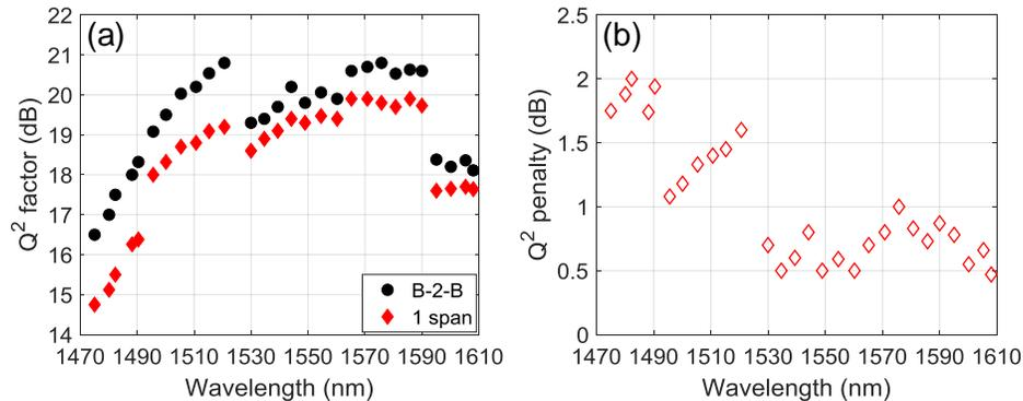
Fig. 3. (a) Comparison of  $Q^2$  factors at different wavelengths between B-2-B and single span measurements and (b)  $Q^2$  penalties vs wavelengths.
