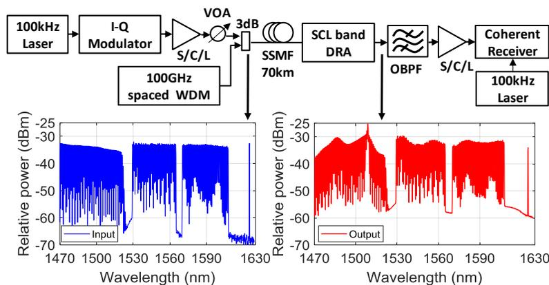
Fig. 2. Coherent transmission experiment setup showing the input spectrum to the span and output spectrum from the DRA.
