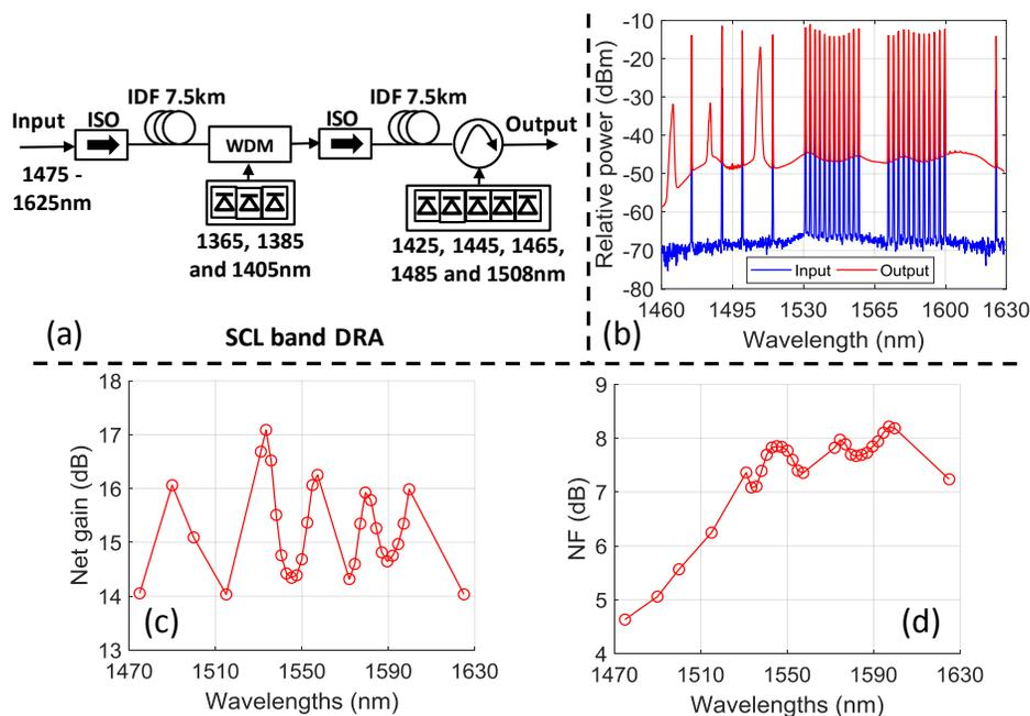
Fig. 1. (a) Schematic diagram of dual-stage DRA; (b) input and output spectra; (c) net gain and (d) noise figure (NF) characteristics.
