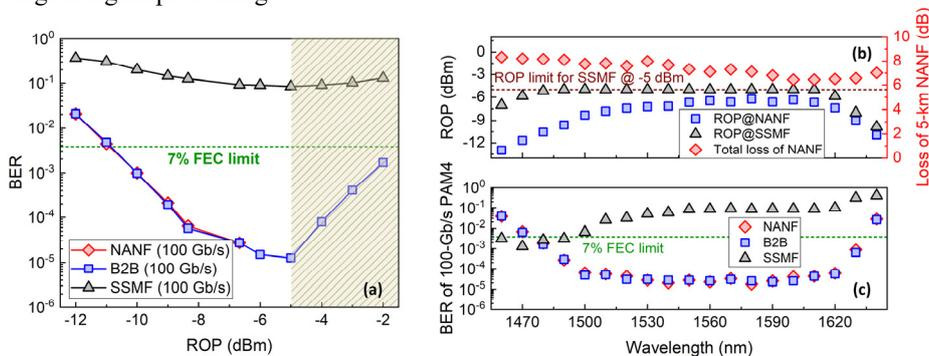
Fig. 2. (a) BER versus ROP at 1550 nm for the 100-Gb/s PAM4, and wavelength sweeping over S+C+L-bands: (b) ROP in different cases and measured total loss of the  $\sim 5$ -km NANF, (c) BER versus wavelength of the 100-Gb/s PAM4.
