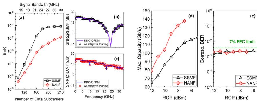
Fig. 3. Comparison between the SSMF and NANF using DDO-OFDM at 1550 nm: (a) BER versus number of data subcarriers; SNR profiles after 5-km transmission in (b) SSMF and (c) NANF; (d)&(e) comparison of the maximum capacity and the corresponding BER.
