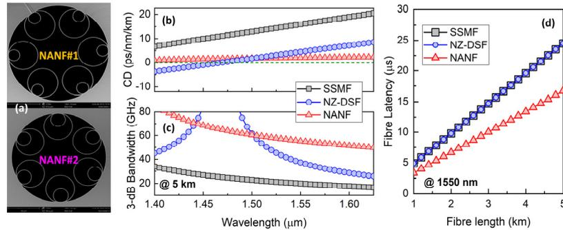
Fig. 1. (a) SEM images of the fabricated NANFs, and comparison amongst the SSMF, NZ-DSF and NANF at a length of 5 km: (b) CD, (c) 3-dB fiber bandwidth, and (d) latency arising from the transmission in the fiber.
