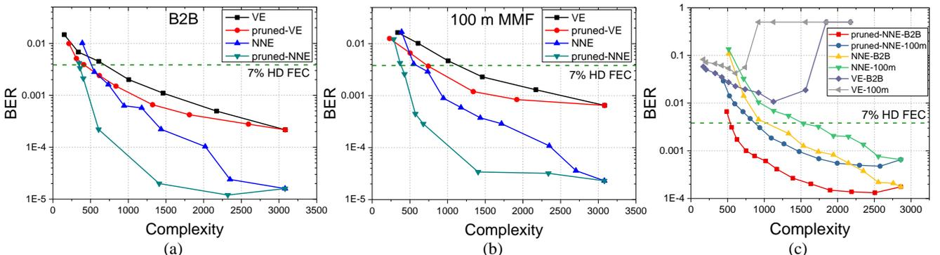
Fig. 2: The efficiency comparison for (a) B2B case and (b) 100-m MMF case at 100-Gbps PAM-4 with pre-distortion. (c) BER as a function of complexity at 112-Gbps PAM-4 without pre-distortion.
