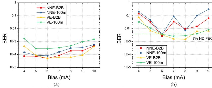
Fig. 3: (a) The BER as a function of VCSEL bias, (b) Pruned equalizers for different bias cases.
