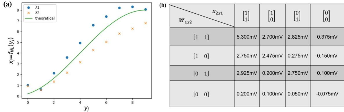
Figure 2. (a) Experimental measurement of modulator nonlinearity, (b) Experimental binary multiplication results with detected voltage values.
