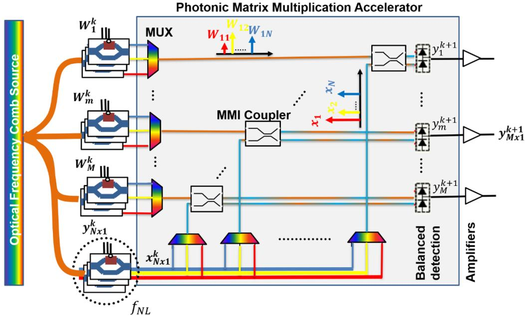
Figure 1. Cascadable analog feed-forward artificial neural network structure with photonic matrix-vector multiplier circuit and Mach-Zehnder modulator nonlinearity.
