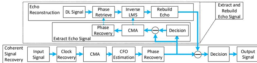
Fig. 2. DSP procedures of echo cancellation. CMA: constant modulus algorithm; CFO: carrier frequency offset; LMS: least mean square
