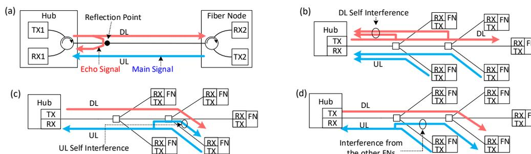
Fig. 1. Echo scenarios in (a) point-to-point (P2P) coherent optical link; (b) DL self-interference; (c) UL self-interference; and (d) UL echo interference from other FNs. DL: downlink, UL: uplink, FN: fiber node, TX: transmitter, RX: receiver.
