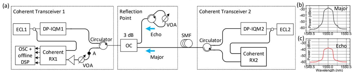
Fig. 3. (a): experimental system diagram; (b): optical spectrum of major signal at A; and (c) optical spectrum of echo signal at A. ECL: external cavity laser; OC: optical coupler; VOA: variable optical attenuator; DP-IQM: dual polarization IQ modulator.
