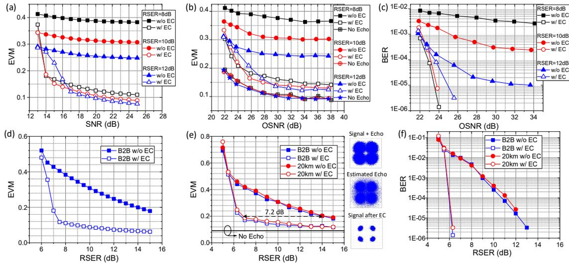
Fig. 4. (a): simulated EVM versus SNR; (b): measured EVM versus OSNR; (c): measured BER versus OSNR; (d): simulated EVM versus RSER; (e) measured EVM versus RSER; and (f) measured BER versus RSER. RSER: received signal to echo ratio.
