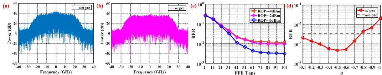
Fig. 2 (a) Received signal spectrum without pre-equalization; (b) Received signal spectrum with pre-equalization; (c) BER versus FFE taps for OBTB transmission without pre-equalization; (d) BER versus  $\alpha$  for pre-equalization at received optical power (ROP) of 0 dBm.
