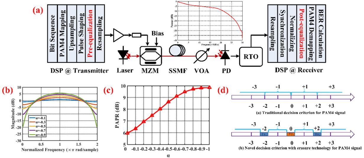
Fig. 1 (a) Experimental setup of C-band 112-Gb/s PAM4 system; (b) Frequency response of pre-filter with different  $\alpha$ ; (c) Signal PAPR after pre-filter with different  $\alpha$ ; (d) Traditional and novel decision criterion for PAM4 in modified FFE-DFE.
