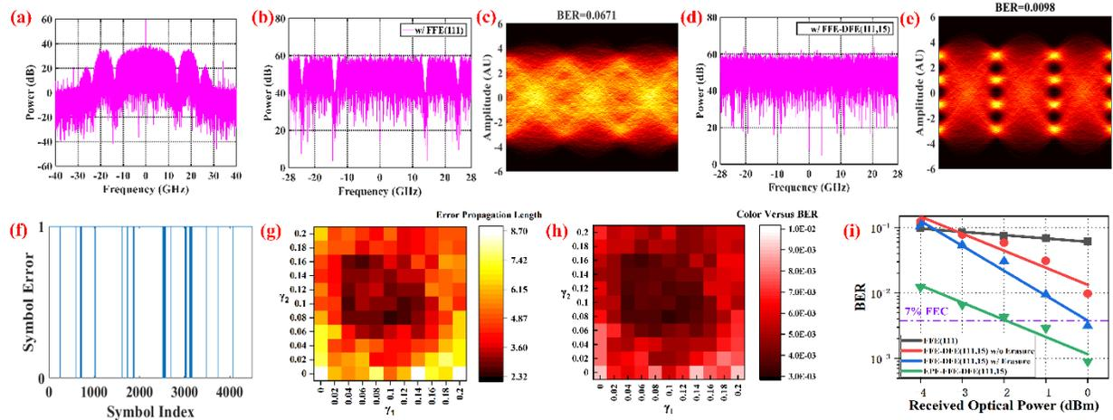
Fig. 3 (a) Received signal spectrum after 20-km transmission; (b-e) Recovered signal spectrums and eye diagrams with FFE and FFE-DFE, respectively; (f) Symbol error with FFE-DFE; (g-h) Error propagation length and BER with different erasure factors; (i) BER versus ROP with different equalizations.
