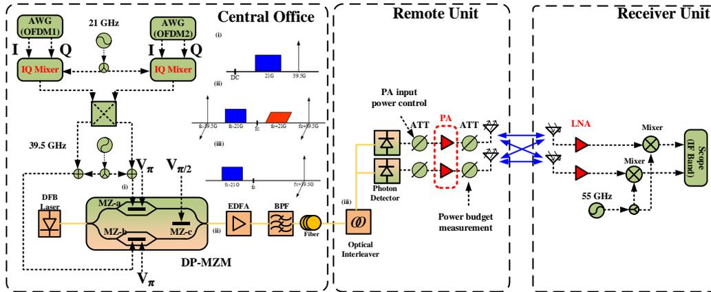
Fig. 3. Experiment setup V-Band RoF system with Volterra compensation.
