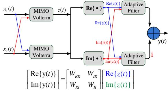
Fig. 2. Functional diagram of I/Q Volterra filter
