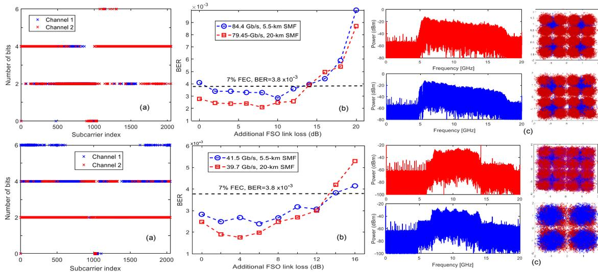
Fig. 3. Performance of  $2 \times 2$  MIMO signal over the seamless fiber-FSO system in the DL (upper) and UL (lower).
