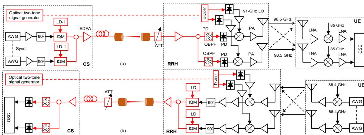
Fig. 2. Experimental setup for  $2 \times 2$  MIMO mmWave signal transmission over seamless fiber-FSO system: (a) DL, (b) UL.
