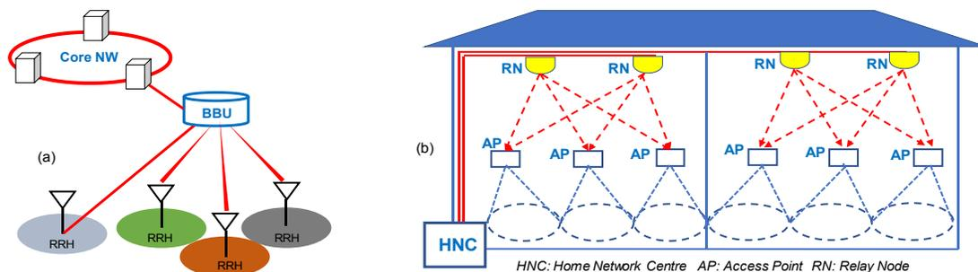
Fig. 1. (a) Seamless fiber-FSO system for mmWave signals; (b) cascaded fiber-FSO-mmWave for ultrahigh-speed access.
