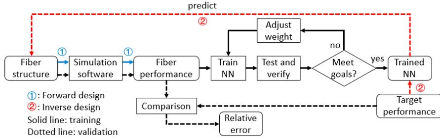
Fig. 1. Flow chart of the proposed NN assisted inverse design method.
