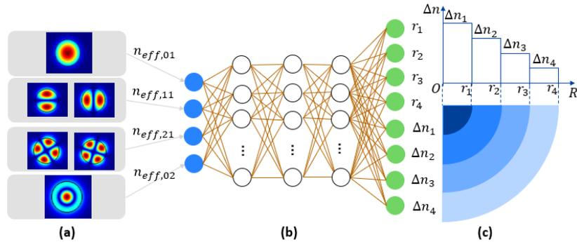
Fig. 2. The inverse design frame of NN. (a) The four modes (mode groups for LP11 and LP21); (b) NN structure; (c) 4-ring FMF structure
