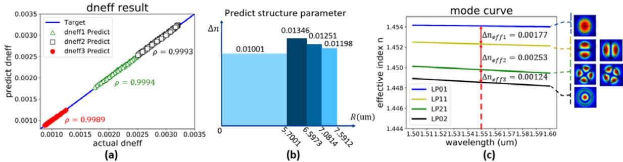
Fig. 3. (a) Correlation diagrams between actual and predict data to evaluate the design accuracy. (b) The predicted FMF structural parameter. (c) The predicted dispersion curve and field diagrams for the four modes.
