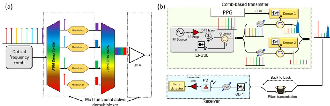
Figure 1: (a) Generic architecture of comb-based WDM transmitter system (dotted boxes show the functions realised by the active demultiplexer). (b) Experimental setup of the proposed comb-based transmission system. Here, VOA: variable optical attenuator, PPG: pulse pattern generator, PD: photodetector, OBPF: optical band pass filter, ED: error detector.
