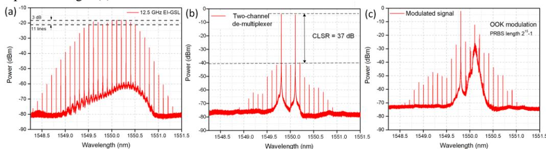
Figure 2: Optical spectra of (a) EI-GSL with FSR of 12.5 GHz, (b) combined demultiplexers output without data modulation and (c) combined demultiplexers output with modulated Demux 1. OSA resolution: 20 MHz, spectra (b) & (c) recorded with 5 dB attenuation before the OSA
