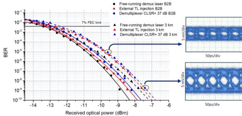
Figure 3: BER vs. received optical power: solid and dotted lines correspond to B2B and 3 km fiber transmission respectively. Insets are eye diagrams recorded at the indicated BERs.
