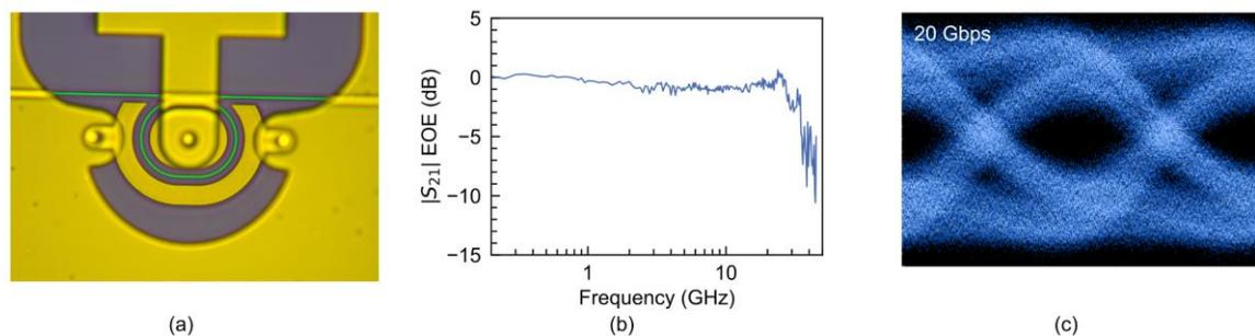
Fig. 3. (a) BTO-Si ring modulator. (b) Bandwidth measured in low-Q ring modulator. (c) Eye diagrams of modulated signal from ring modulator. Data was transmitted at 20 Gbps using a source voltage of 1 V to drive the modulator.
