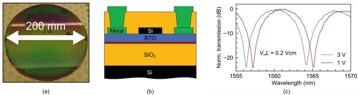
Fig. 2. (a) Wafer bonding of BTO layers using 200mm substrate wafers. (b) Schematic cross-section of the BTO devices fabricated on silicon substrates. (c) Tuning of BTO Mach-Zehnder modulator showing a  $V_\pi L$  of just 0.2 Vcm.
