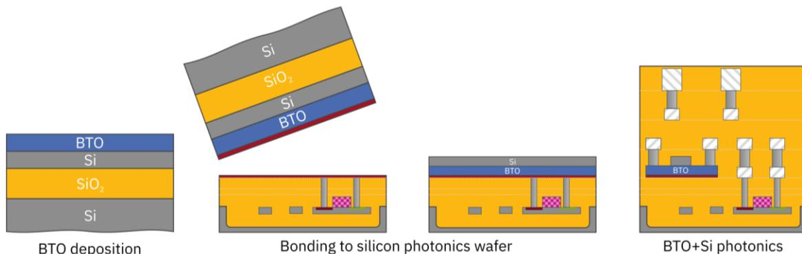
Fig. 1. Concept for integration of BTO with silicon photonics using molecular wafer bonding. BTO is deposited on an SOI wafer and can then be bonded to any wafer with electronic or photonic structures at a planarized level. The donor wafer is removed using mechanical and chemical processes. BTO devices can then be processed along with any back-end-of-line process steps.
