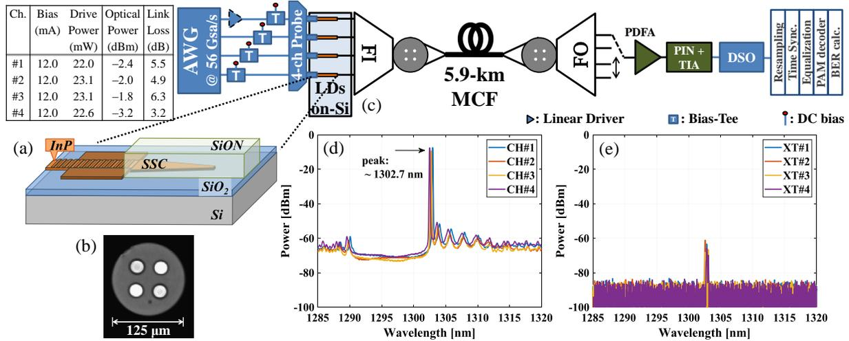
Fig. 1: (a) Membrane DML-on-Si structure, (b) Cross-section of 125- $\mu\text{m}$  cladding four-core MCF, (c) Experimental setup and parameters, (d) Lasing spectra, and (e) optical XT after fan-in.
