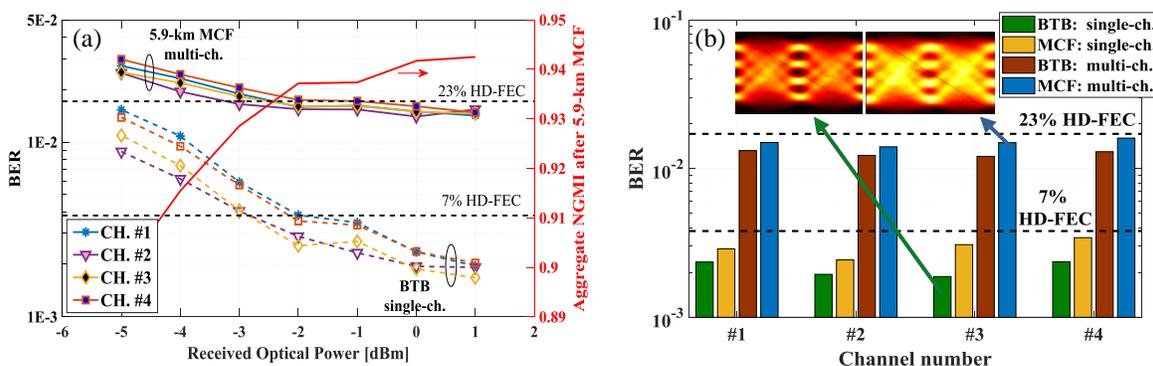
Fig. 2: (a) BER vs. ROP results, (b) dependency of BER on channel operation at ROP = 0 dBm; inset: equalized eye diagrams for channel #3 after single-channel BTB (left) and multi-channel 5.9-km MCF (right) transmissions.
