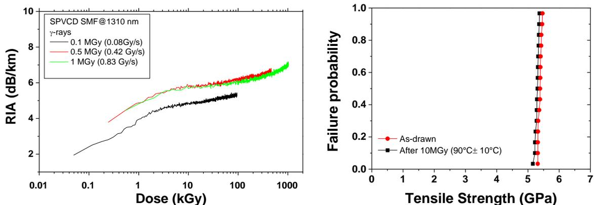
Fig. 2. left)  $\gamma$ -ray RIA at 1310 nm (RT) in radiation hardened SPCVD SMF [8] right) Tensile strength versus failure probability before/after 10 MGy( $90^\circ\text{C}$ ) irradiation of a polyimide coated fiber (see [8] for more details).
