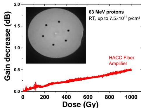
Fig. 3. Radiation induced gain decrease in an EDFA (gain of 27 dB before irradiation) designed with a HACC Erbium doped fiber (loaded with D<sub>2</sub>) under 63 MeV proton exposure up to  $7.5 \times 10^{11}$  p/cm<sup>2</sup> a t RT.
