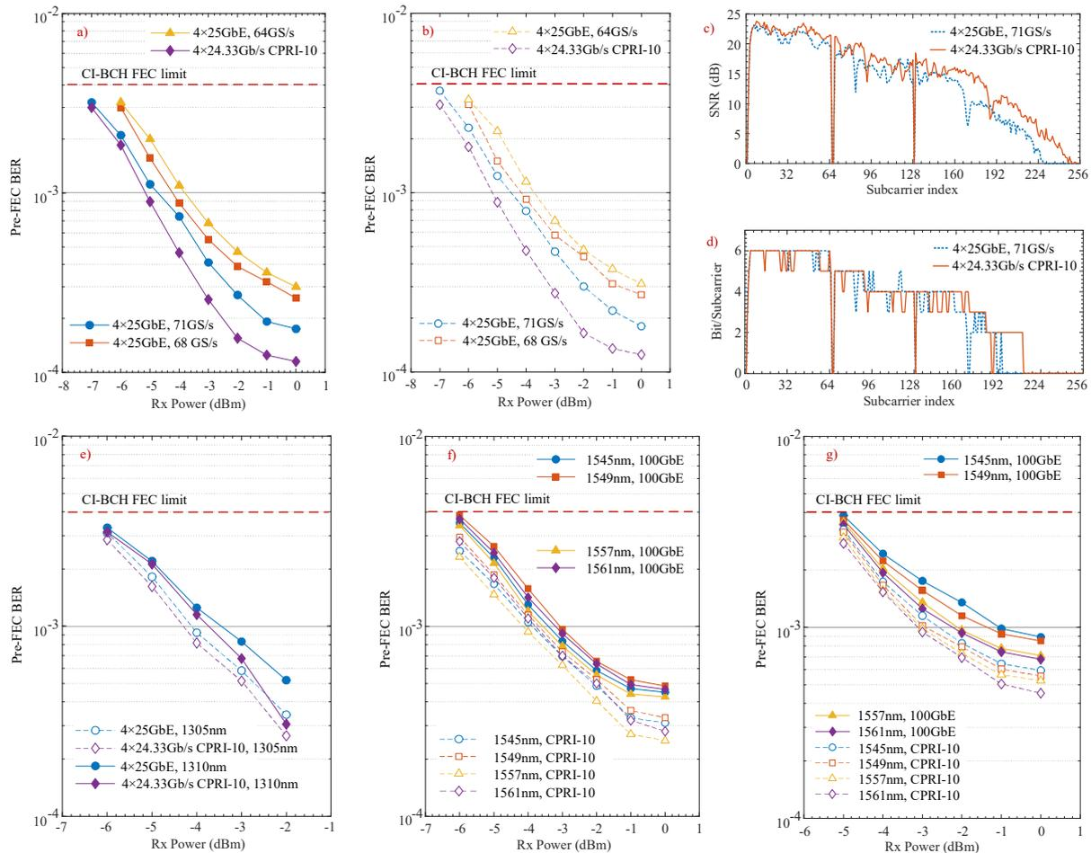
Fig. 4. Overall experimental results including a-b) – B2B sensitivities of 1310nm and 1305nm channels, respectively; c-d) SNR and allocated bits per subcarrier for the 1310nm channel at 0dBm of Rx power; e) – Performance over 20km of 200Gb/s O-band; g) – B2B sensitivities and transmission performance over 20km of 400Gb/s C-band DWDM system.
