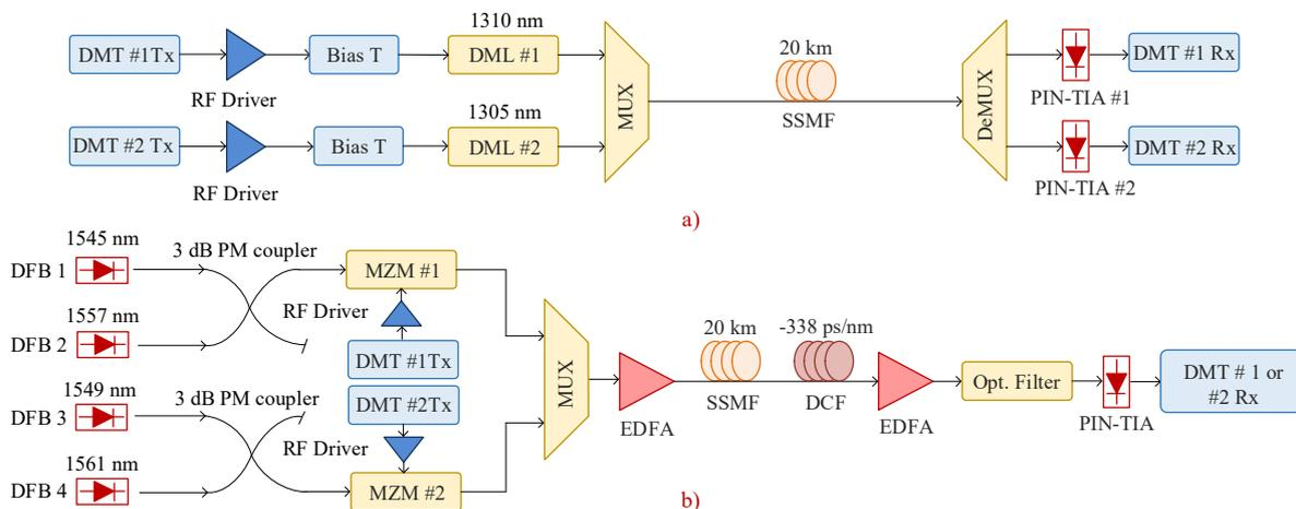
Fig. 3a) – Real time O-band, amplifier-less, LAN-WDM2 200Gb/s transmission setup supporting  $8 \times 25\text{GbE}$  Ethernet or  $8 \times 24.33\text{Gb/s}$  CPRI-10 traffic over 20km; b) – Real time C-band DWDM 400Gb/s transmission setup supporting  $16 \times 25\text{GbE}$  Ethernet or  $16 \times 24.33\text{Gb/s}$  CPRI-10 traffic over 20km; DCF – dispersion compensating fibre.
