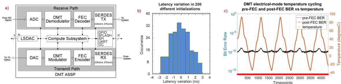
Fig. 2a) – Block diagram of the 16nm CMOS ASIC; b-c) – Latency variation and temperature dependency measurements of the ASIC
