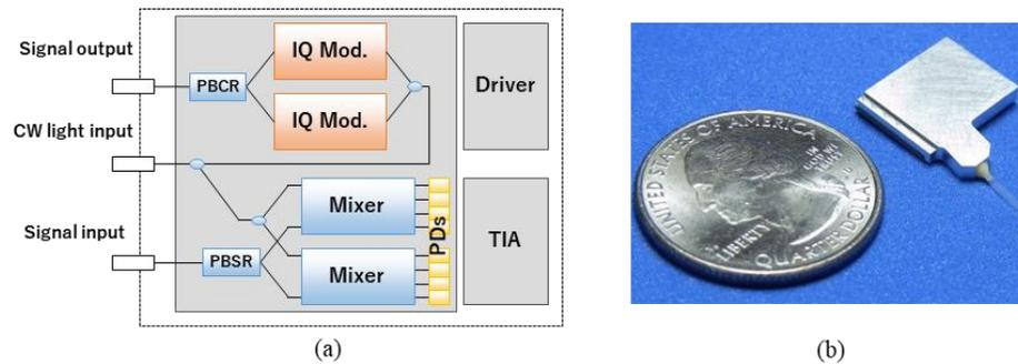
Figure 1. (a) Schematic configuration and (b) picture of fabricated COSA
