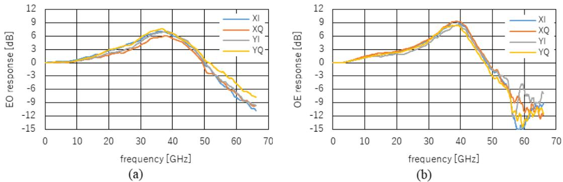
Figure 2. (a) EO responses of transmitter side and (b) OE responses of receiver side
