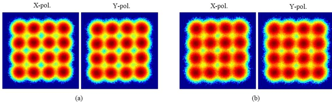
Figure 3. (a) 80 Gbaud and (b) 96 Gbaud polarization multiplexed 16QAM constellations
