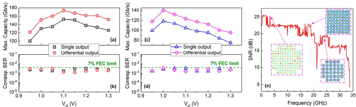
Fig. 3. Maximum capacity and the corresponding BER versus  $V_{ct}$  of the adaptively-loaded DMT transmission: (a)&(b) B2B link, (c)&(d) 2-km SSMF link; (e) SNR profile of the DMT transmission using the differential output in the B2B link with  $V_{ct}$  being 1.1 V.
