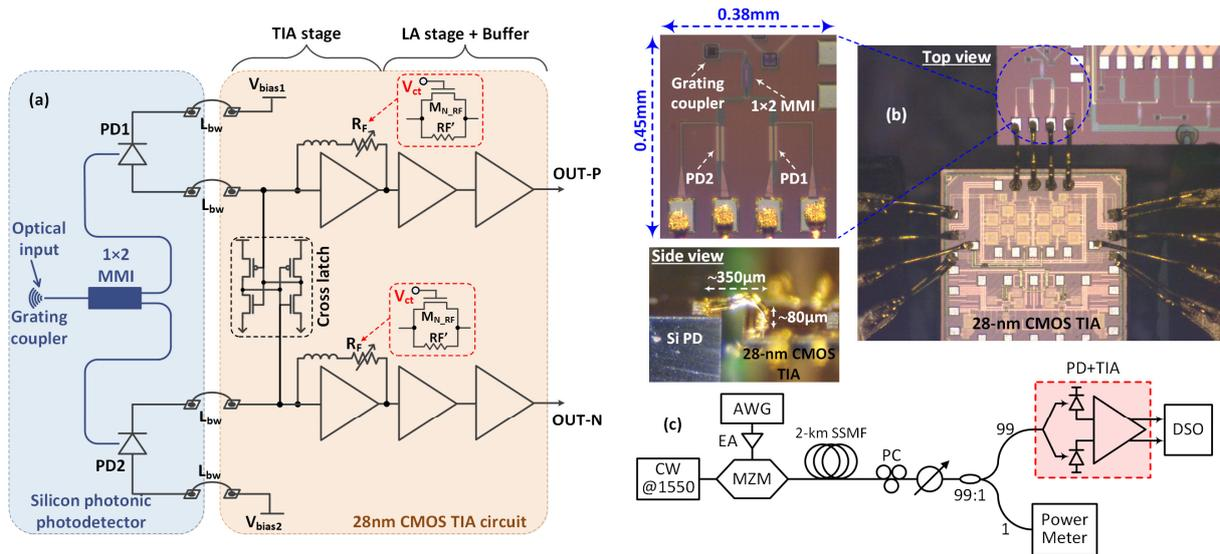
Fig. 1. (a) Block diagram of the proposed integrated optical receiver, (b) microscope view of the wire-bonded photodetector and TIA, and (c) experimental setup of the transmission system.
