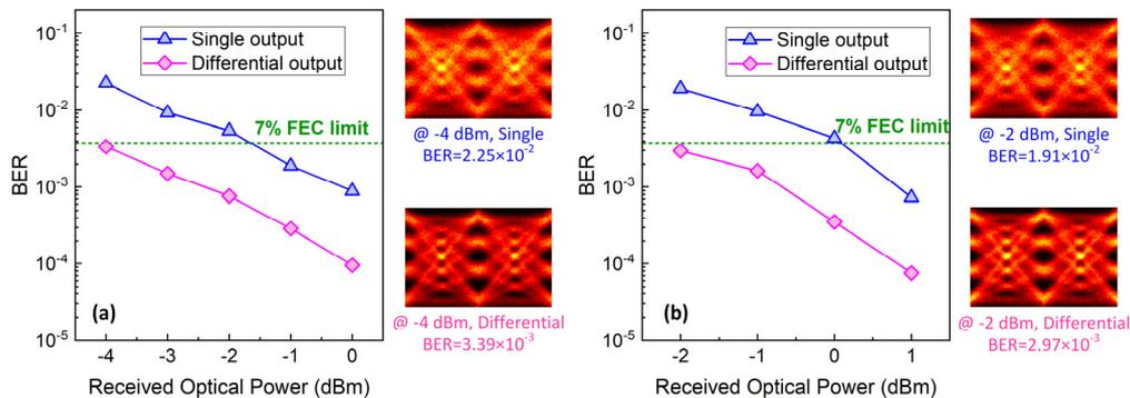
Fig. 2. BER versus ROP for 100-Gb/s PAM4 transmission: (a) B2B link, and (b) 2-km SSMF link.
