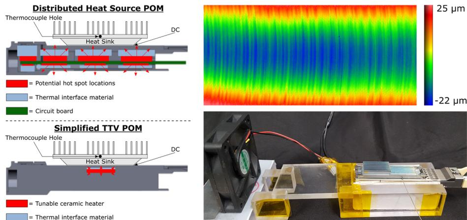
Fig. 2. Distributed heat source POM (top left), s-TTV-POM (bottom left); sample HS surface profile (top right) and s-TTV setup (bottom right).
