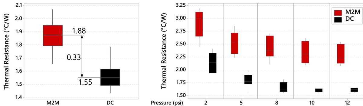
Fig. 3. Boxplot of TR using M2M (in red) and DC-POM (in black) interfaces measured for  $\sim 100$  HS (left). Data boxplot for TRs at the M2M (in red) and DC-POM (in black) interfaces after 10 I&Ps with increasing contact pressure between the HS and s-TTV-POM (right).
