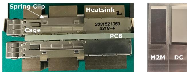
Fig. 1. Side view of QSFP-DD POM, cage, and spring clip assembly (left). Heat sinks with durable coating (DC) and without (M2M) (right).
