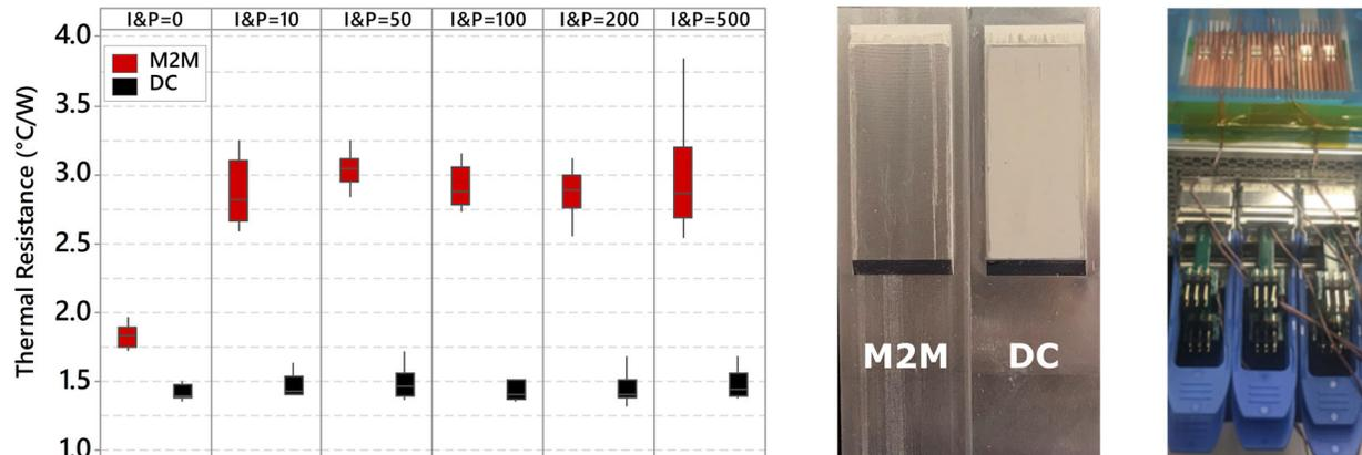
Fig. 4. Boxplot of TR on s-TTV for M2M (in red) and DC (in black) after 0 to 500 I&Ps (left). Example of 50 I&P damage on both HS surfaces (center). Setup / configuration for one of Juniper Networks performance verification tests (right).
