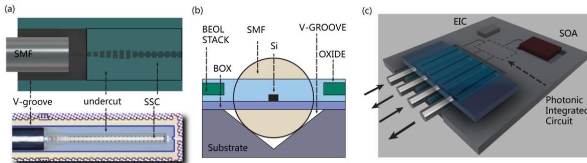
Fig. 1. (a) Schematic and microscope top view of an metamaterial edge coupler with V-groove and fiber attach. (b) Cross-sectional diagram of the edge coupler with V-groove at the fiber interface. (c) Schematic of the PIC chip package with attached single-mode fiber array, the cover, optical source, and the attached electric chip. SMF: single-mode fiber, SSC: spot size converter, BEOL: back-end-of-line, SOA: semiconductor optical amplifier, EIC: electric integrated circuits.
