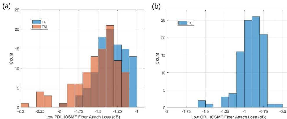
Fig. 3. Sampling fiber-attach insertion loss data. (a) Statistic data of insertion loss of IOSMF design with low polarization-dependent loss, (b) statistic data of insertion loss of IOSMF design with low optical return loss. A total of 100 samples for each design were picked randomly, over 4 lots and 8 wafers. The test was done with several cleaved single-mode fibers under IPA index match condition.
