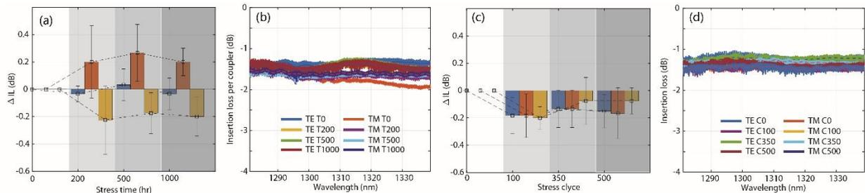
Fig. 4. Fiber-attach package reliability assessment. (a) IL variation and (b) corresponding spectra with damp heat stress test over 200, 500, and 1000 hours, (c) IL variation and (d) corresponding spectra deep thermal cycle stress test over 100, 350 and 500 cycles.
