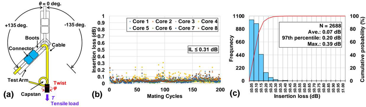
Fig. 3. (a) Jumper test facility for the mechanical tests, (b) the IL variation during the durability test for 1 pair of the fabricated connectors, and (c) the IL histogram for the random mating test (Sample size 2688 = 112 random connection pairs  $\times$  3 mating cycle  $\times$  8 cores).
