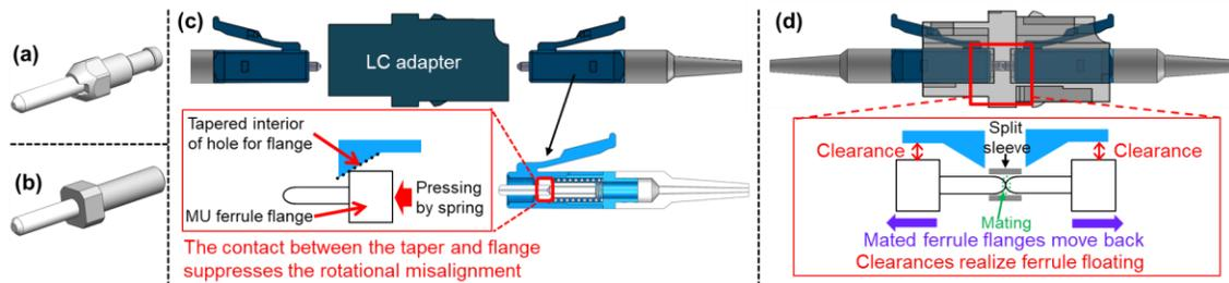
Fig. 2. Schematics of standard (a) LC and (b) MU ferrule flanges with the identical ferrule diameter, and (c) unmated and (d) mated LC-interface MCF connectors with the proposed housing with tapered hole for a standard MU flange. When the connectors are unmated, ferrule flange is precisely rotationally aligned by the taper. When the connectors are connected, ferrule can be floating by the clearance.
