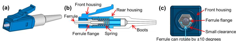
Fig. 1. (a) Appearance, (b) cross section, and (c) clearance between the ferrule flange and the housing of the conventional LC connector.
