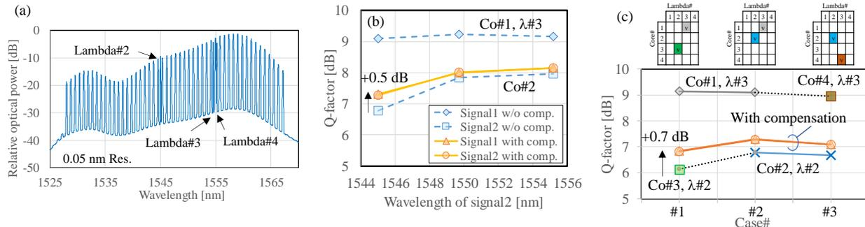
Fig. 4. Experimental results of cross-SDM/WDM Q-difference compensation scheme for 192-km MCF transmission, a) an optical spectrum of core-path#1 after 192-km transmission, b) Wavelength dependency of Q-factor with/without application of the scheme after 192-km MCF transmission, c) SDM/WDM signal combination cases and compensation results.
