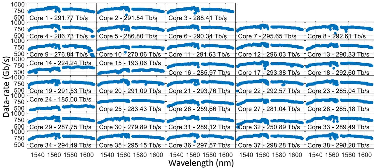
**Fig. 3:** Data-rates after implemented LDPC + HD-FEC coding scheme for all wavelength channels of all cores. Data-rates in each plot after the implemented de-coding scheme.
