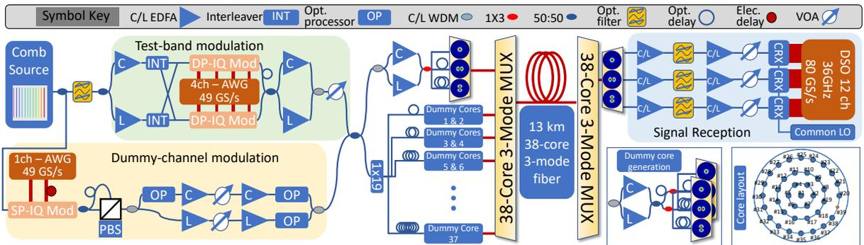
Fig. 1: Experimental setup for C+L-band transmission in a 38-core 3-mode fiber.
