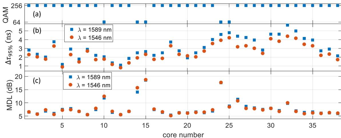
**Fig. 2:** (a) Transmitted QAM-order for all 38 cores. (b) Impulse response length ( $\Delta\tau_{95\%}$ ) and (c) mode-dependent loss (MDL) of two different WDM channels for all 38 cores
