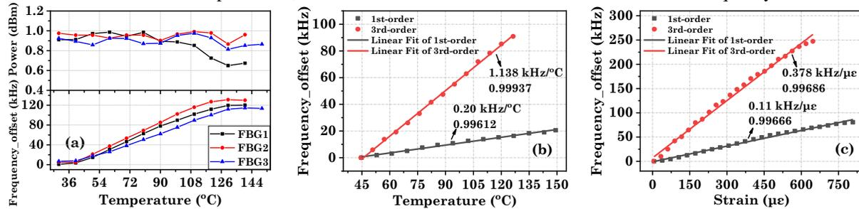
Fig. 4. (a) Peak power and frequency offset vs. temperature for the heated FBG<sub>1</sub>, FBG<sub>2</sub>, and FBG<sub>3</sub>. The linearity and sensitivity of the 1st-order and the 3rd-order oscillating signals for FBG<sub>3</sub> (b) at different temperatures and (c) at different strains.
