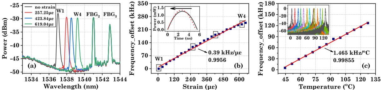
Fig. 3. (a) Reflection spectra and (b) frequency offset of the oscillating signal vs. strain for the stretched FBG<sub>1</sub>. Inset: Time domain waveforms before and after stretching. (c) Frequency offset vs. temperature for the heated FBG<sub>2</sub>. Inset: Oscillating waveforms at different temperatures.
