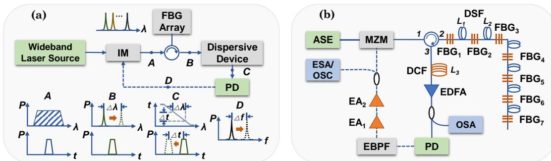
Fig. 1. (a) Schematic diagram and (b) experimental setup of the proposed method.
