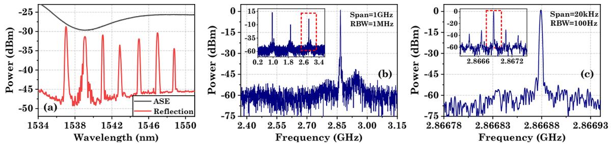
Fig. 2. (a) Reflection spectrum of the FBG sensor array. Electrical spectrum of the 2.868 GHz oscillating signal in the multiloop OEO when (b) span = 1 GHz, RBW = 1 MHz (c) span = 20 kHz, RBW = 100 Hz.
