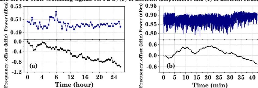
Fig. 5. Time stability with (a) the stretched FBG<sub>1</sub> at the room temperature; (b) the heated FBG<sub>3</sub> at the fixed strain.
