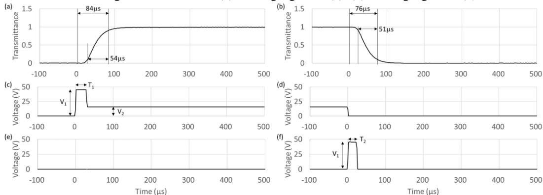
Fig. 3. Switching waveforms with revised driving. (a) Optical output changing from OFF to ON. (b) Optical output returning from ON to OFF. (c) 1st heater driving signal of (a). (d) 1st heater driving signal of (b). (e) 2nd heater driving signal of (a). (f) 2nd heater driving signal of (b).
