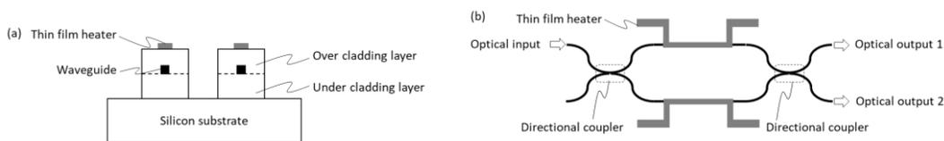
Fig 1. (a) Structure of a silica-based PLC device. (b) Configuration of a switching element.
