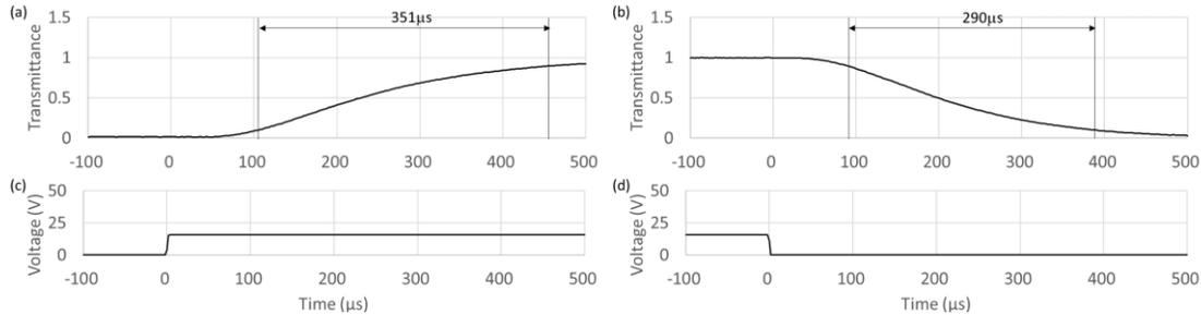
Fig. 2. Switching waveforms with standard driving. (a) Optical output changing from OFF to ON. (b) Optical output returning from ON to OFF. (c) Driving signal of (a). (d) Driving signal of (b).
