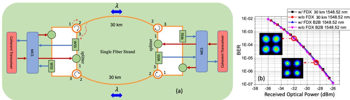
Fig. 3. Full-duplex system setup (a) and experimental results (b), BER: bit error rate.
