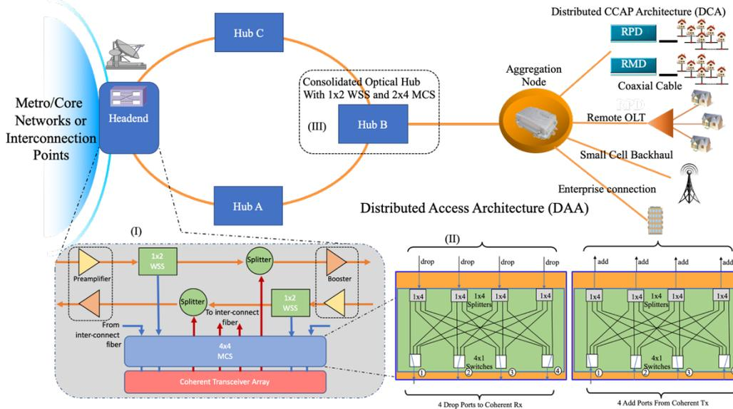
Fig. 1. Architecture design of inter-hub network with CDC functions.
