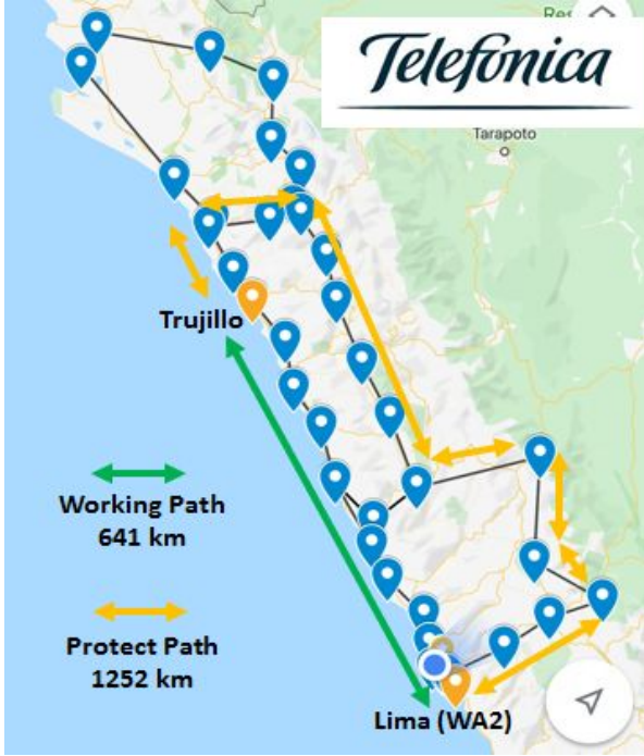
Fig. 1: Bi-directional transmission: working and protection fiber
