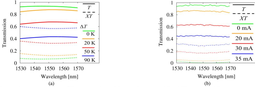
Fig. 3 (a) Calculated transmission ( $T$ ) and  $XT$  spectra for 0 K to 90 K. (b) The measured  $T$  and  $XT$  spectra for different injection currents of the fabricated mode divider.
