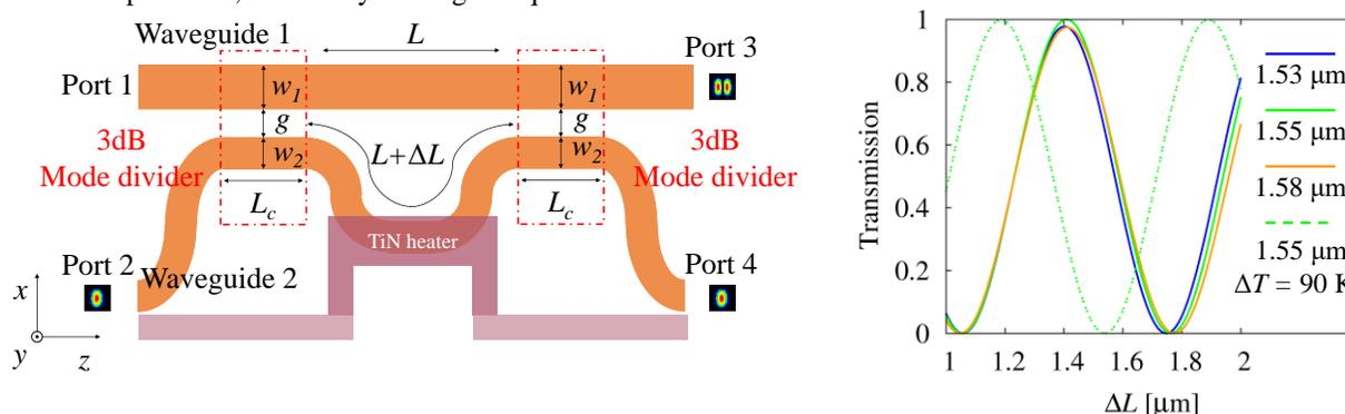
Fig. 1 (a) The schematic of a mode divider with arbitrary branching ratio based on multimode WINC. (b) Transmission (port2 to port3) as a function of  $\Delta L$  for  $L = 20$  μm.
