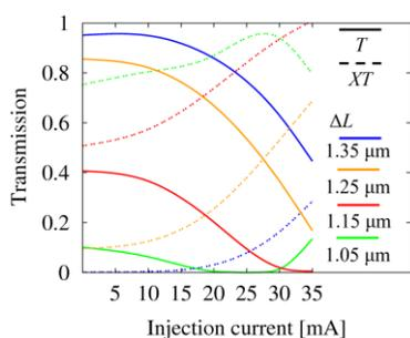
Fig. 4 The measured  $T$  and  $XT$  as a function of the injection current at  $\Delta L = 1.05$  to  $1.35 \mu\text{m}$  for the wavelength of  $1.55 \mu\text{m}$
