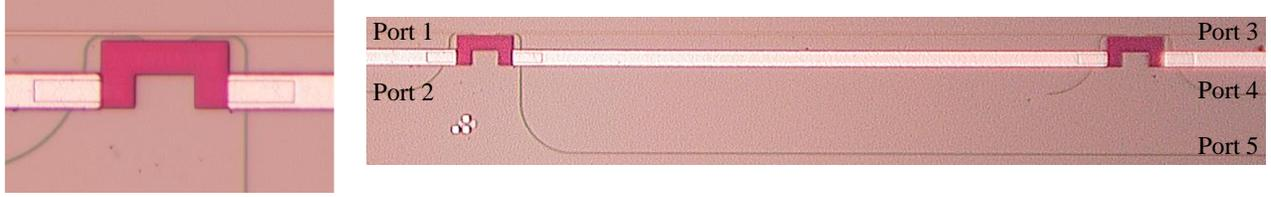
Fig. 2 A micrograph of (left) the fabricated mode divider with arbitrary branching ratio based on multimode WINC and (right) two-cascaded mode divider.
