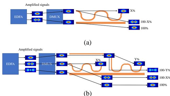
Fig. 5 The concept of mode-gain-equalizer by using the tunable mode divider for (a) two-mode case and (b) three-mode case
