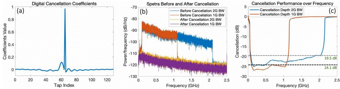
Fig. 2 (a) Digital cancellation coefficients over tap index; (b) self-interference signal spectra before and after SI cancellation; (c) cancellation performance over frequency range.
