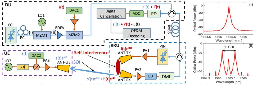
Fig. 1 Experimental setup of the proposed centralized digital cancellation in mm-wave over fiber system; optical spectrum (i) before and (ii) after optical carrier suppression.
