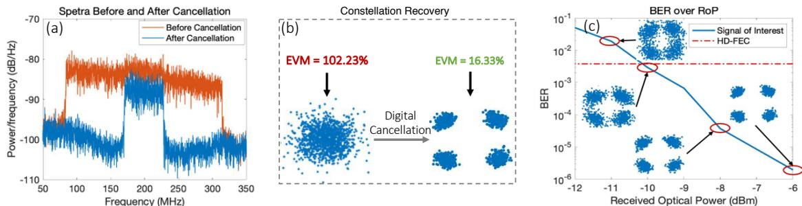
Fig. 3 (a) Interfered signal spectra before and after cancellation; (b) constellation diagrams with and without digital cancellation; (c) BER over received optical power (RoP) at the DU.
